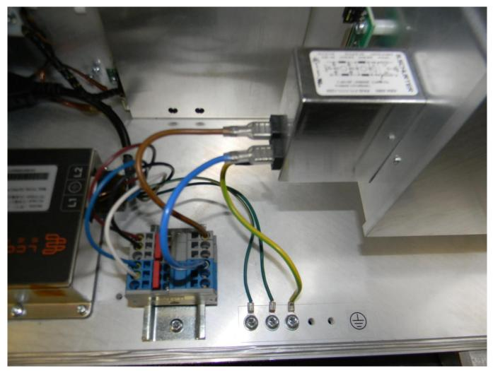
Photo 5: Internal view Chassis Ground
