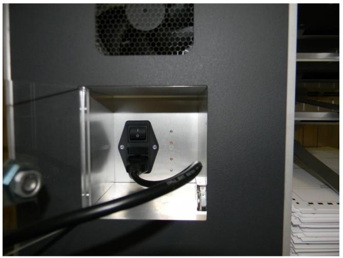
Photo 7: AC inlet/filter module- 2 poles fuse
