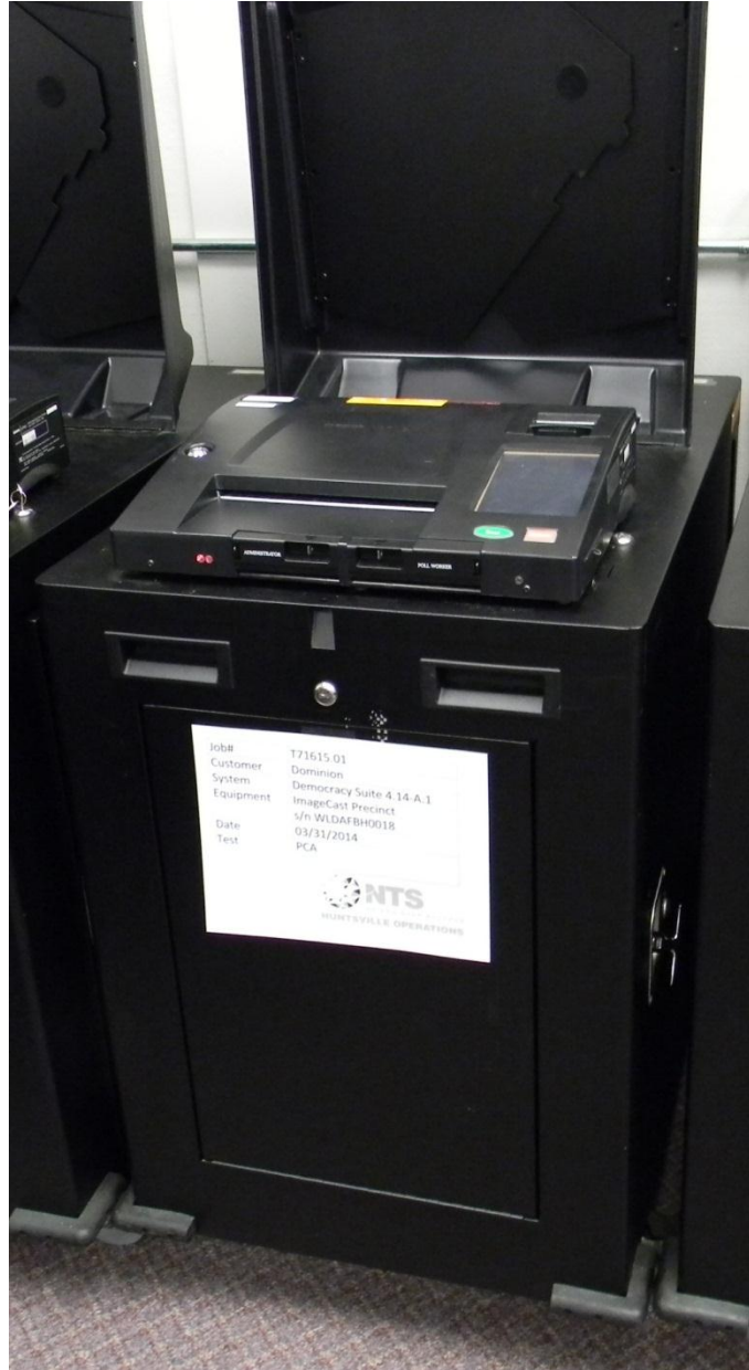
Photograph 2: ImageCast Precinct (ICP) on Metal Ballot Box
