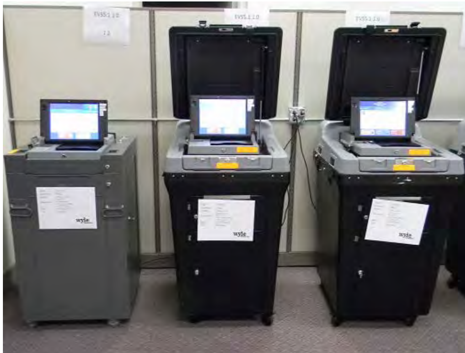
Photograph No. 2 ES&S EVS 5.0.1.0 Accuracy Test Setup
