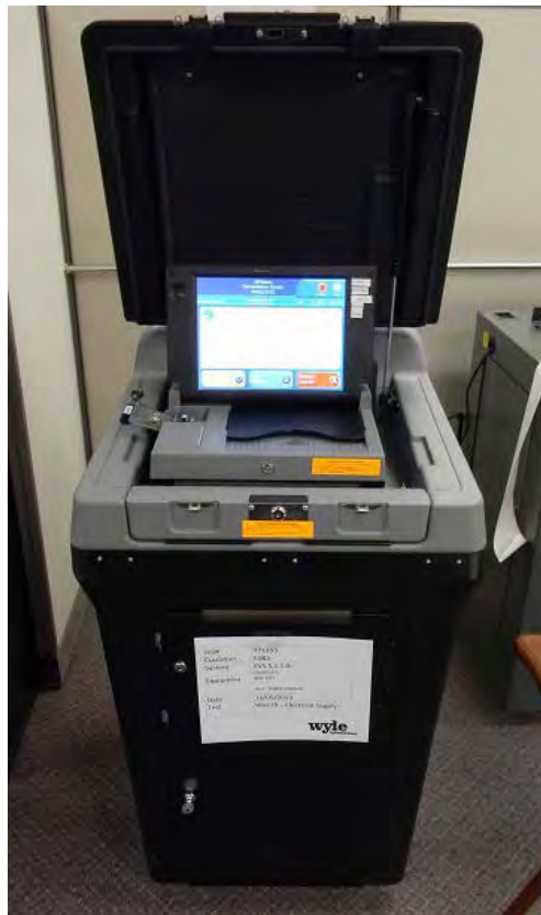
Photograph No. 8 ES&S EVS 5.0.1.0 Electrical Supply Test
