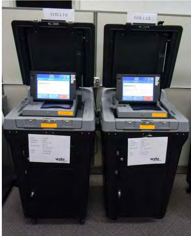
Photograph No. 1 ES&S EVS 5.0.1.0 Functional Test Setup
