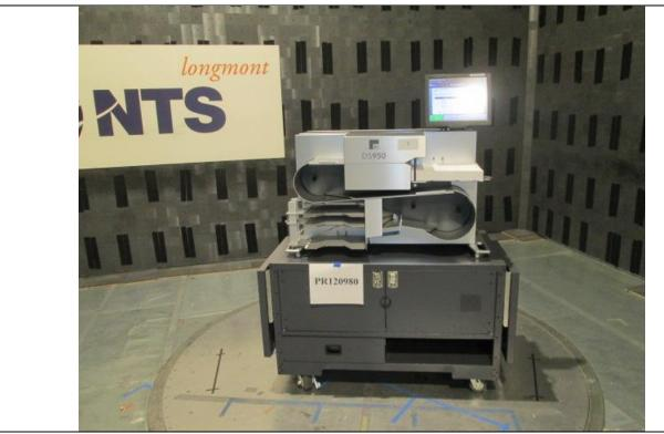
Figure A2: Radiated Emissions Test Setup – Front Side
