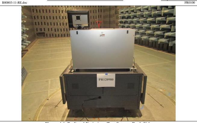
Figure A4: Radiated Emissions Test Setup – Back Side
