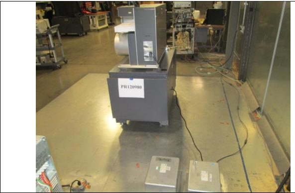
Figure B4: Conducted Emissions Prescan
