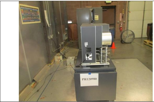
Figure B6: Conducted Emissions Prescan
