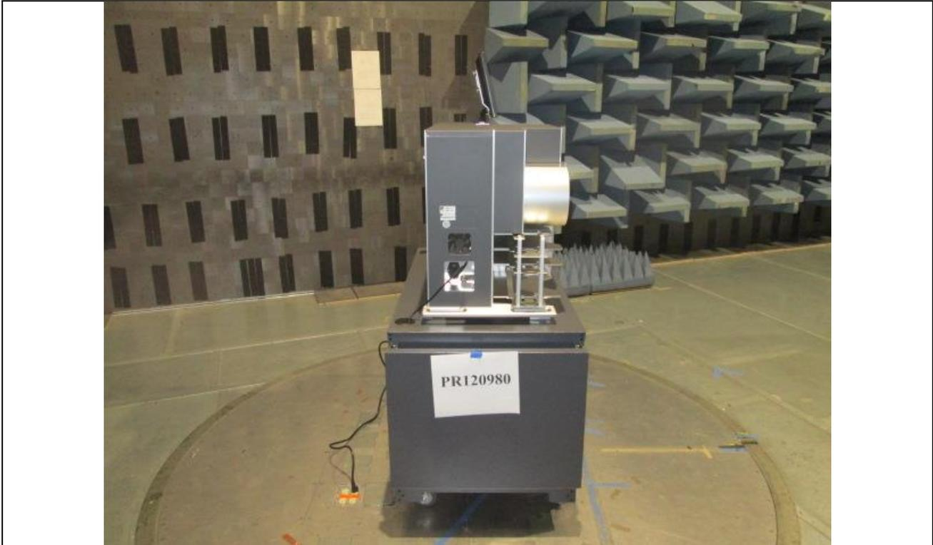
Figure A5: Radiated Emissions Test Setup – Left Side
