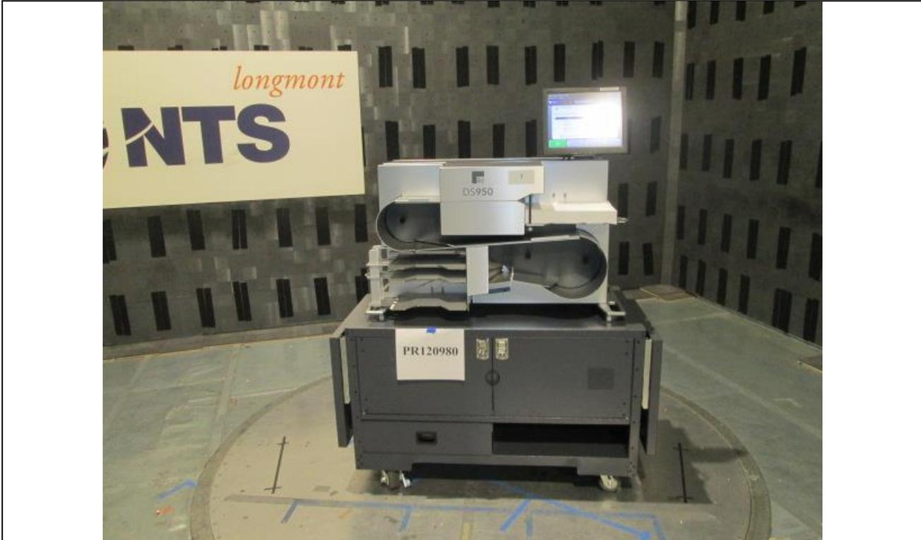
Figure A2: Radiated Emissions Test Setup – Front Side
