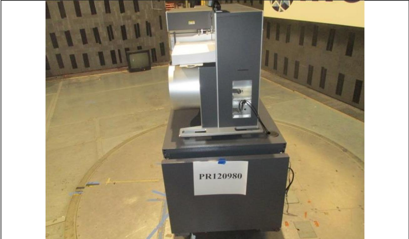
Figure A3: Radiated Emissions Test Setup – Right Side
