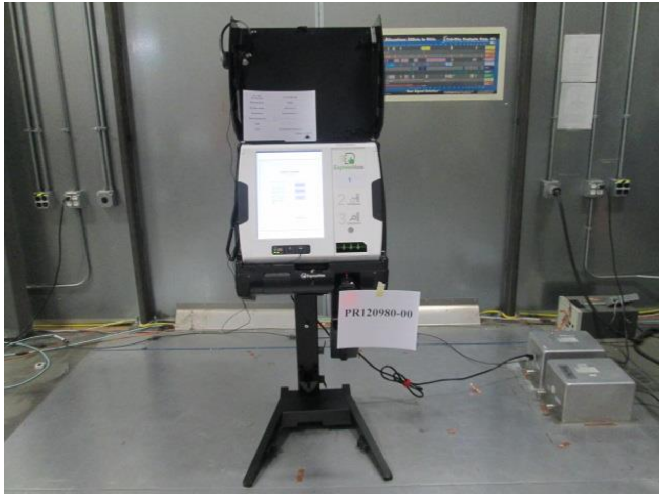
Figure B3: Conducted Emissions Test Setup – Front Side
