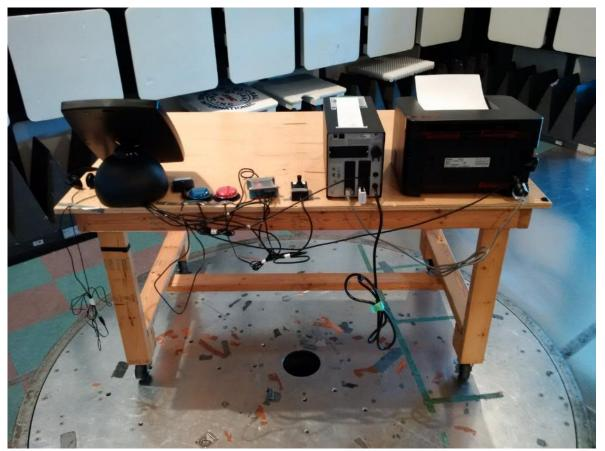
Figure 31 – Radiated Emissions Setup – AVALUE SAMSUNG / SAMSUNG – Photo 1 30MHz – 1GHz
