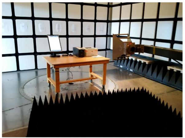
Figure 30 – Radiated Emissions Setup – AVALUE 21" / ICX 21" – Photo 3 1GHz – 10GHz
