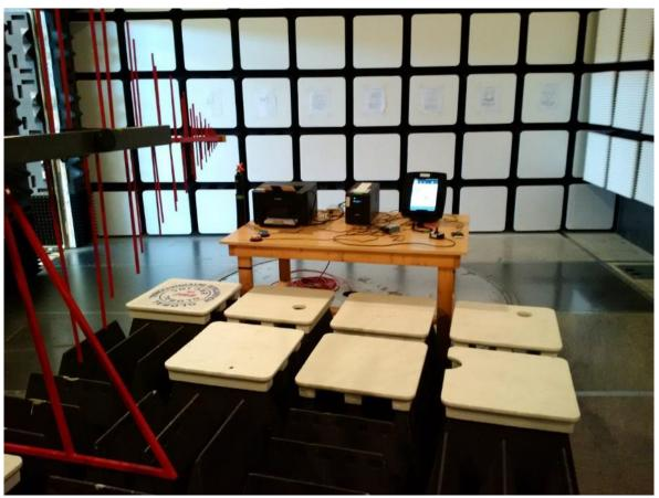
Figure 41 - Electromagnetic Susceptibility Setup AVALUE SAMSUNG / ICX SAMSUNG
