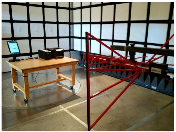
Figure 26 – Radiated Emissions Setup – AVALUE 15" / ICX 15" – Photo 1 30MHz – 1GHz
