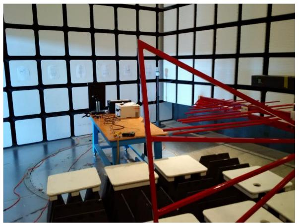
Figure 40 - Electromagnetic Susceptibility Setup - AVALUE 21" / ICX 21"
