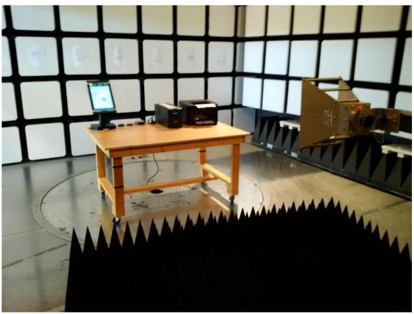
Figure 27 – Radiated Emissions Setup – AVALUE 15" / ICX 15" – Photo 2 1GHz – 10GHz
