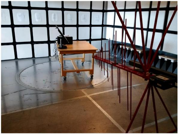
Figure 29 – Radiated Emissions Setup – AVALUE 21" / ICX 21" – Photo 2 30MHz – 1GHz
