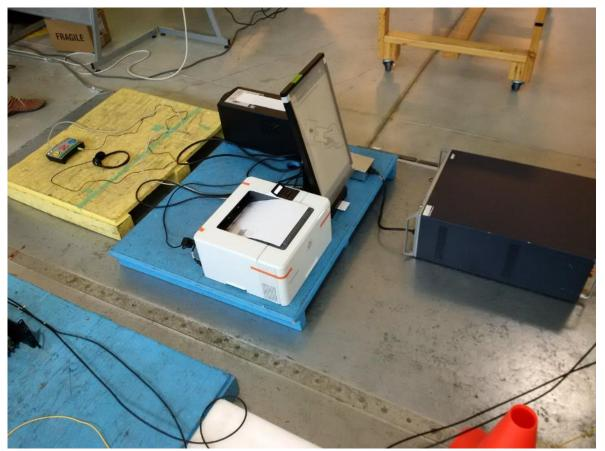
Figure 44 - Electrical Fast Transient, Lightning Surge & Electrical Power Disturbance AVALUE 21" / ICX 21"
