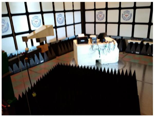
Figure 32 – Radiated Emissions Setup – AVALUE SAMSUNG / SAMSUNG – Photo 2 1GHz – 10GHz
