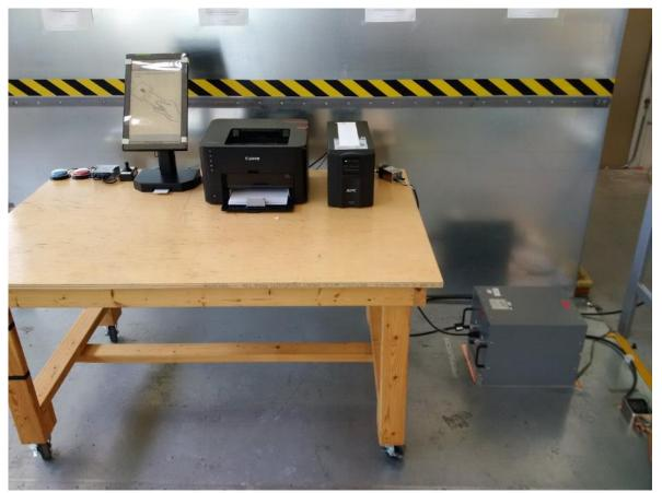
Figure 17 – Conducted Emissions Setup – AVALUE 15" / ICX 15" – Photo 1
