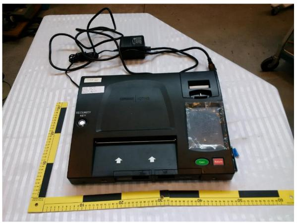
Figure 6 – EUT Close Up PCOS 320C / ICP
