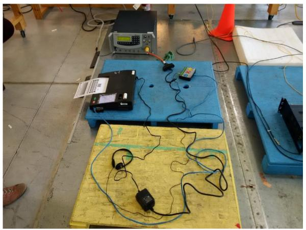
Figure 46 - Electrical Fast Transient, Lightning Surge & Electrical Power Disturbance PCOS 320C / ICP
