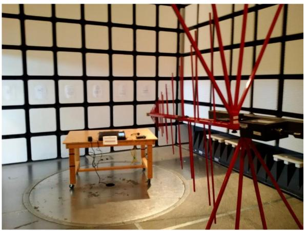
Figure 34 – Radiated Emissions Setup – PCOS 320C / ICP – Photo 2 30MHz – 1GHz
