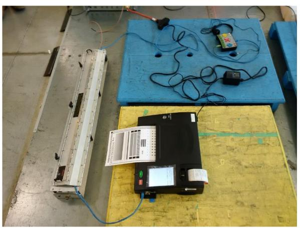
Figure 47 - Electrical Fast Transient PCOS 320C / ICP Ethernet I/O For Headphone Box
