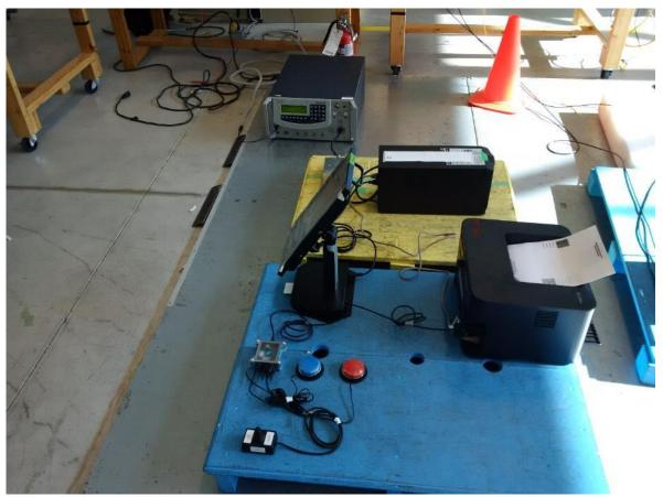
Figure 43 - Electrical Fast Transient, Lightning Surge & Electrical Power Disturbance AVALUE 15" / ICX 15"
