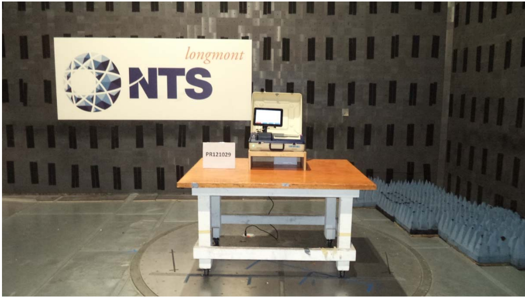
Figure A1. Radiated Emissions Test Setup (Front).
