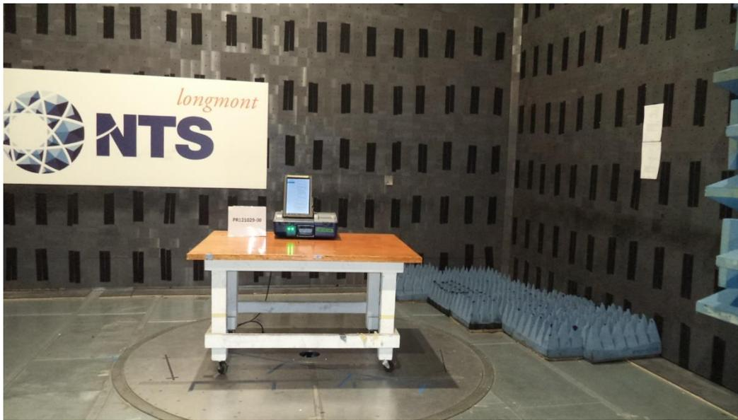
Figure A1. Radiated Emissions Test Setup (Front).
