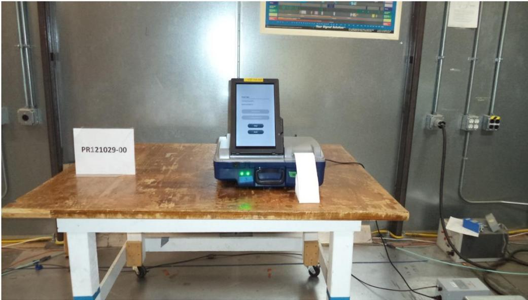
Figure A1. Conducted Emissions Test Setup.
