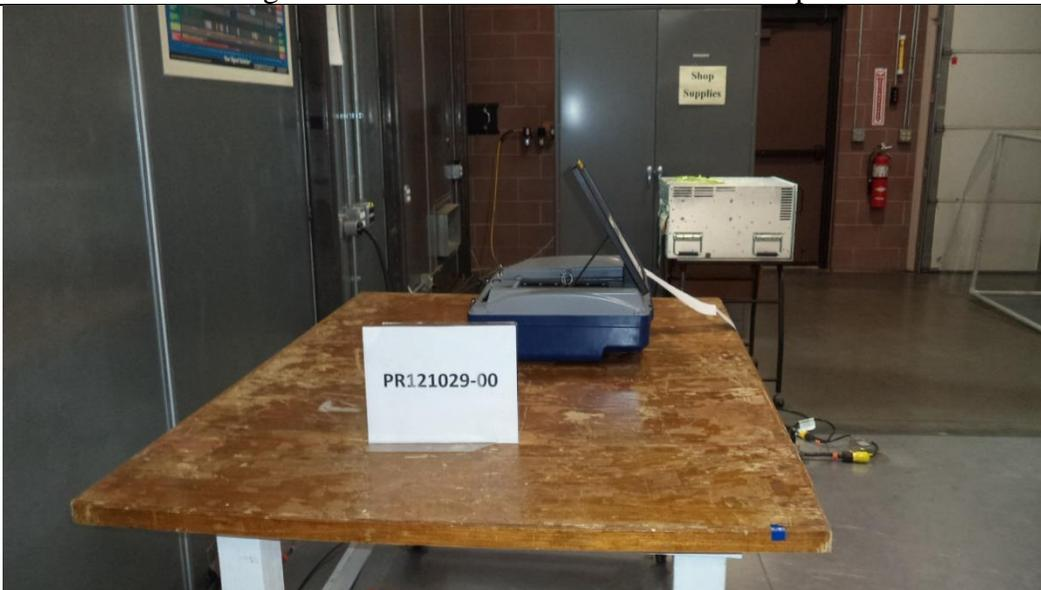
Figure A2. Conducted Emissions Test Setup.
