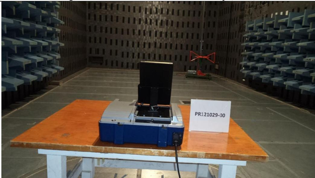
Figure A1. Radiated Emissions Test Setup (Back).
