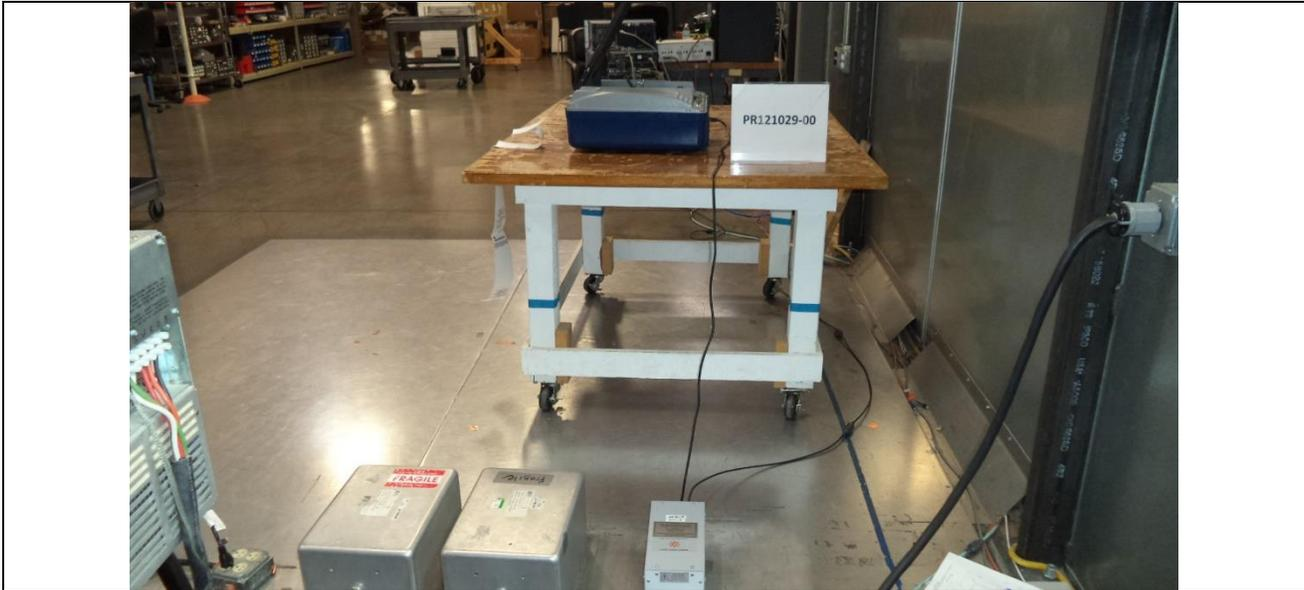
Figure A3. Conducted Emissions Test Setup.
