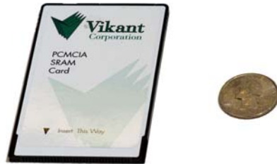
PCMCIA Memory Card for M100 Optical Scanner (compared to the size of a quarter)
