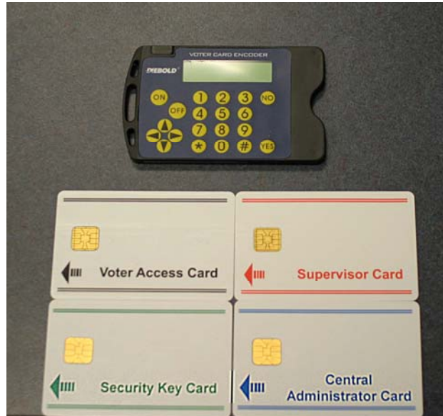
Voter Access and Supervisor Cards used with the Premier DRE Voting System
