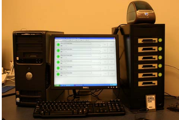
Election Media Processor (EMP) used with the Premier Voting System
