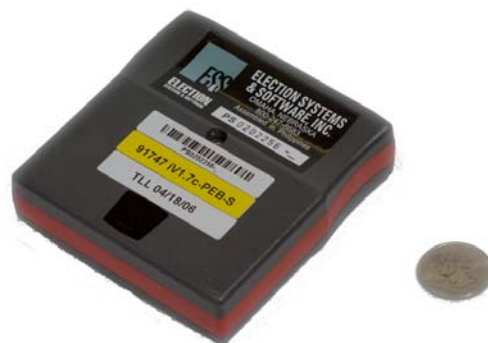
ES&S Personalized Electronic Ballot (PEB) for the iVotronic DRE Voting Machine (compared to the size of a quarter coin)
