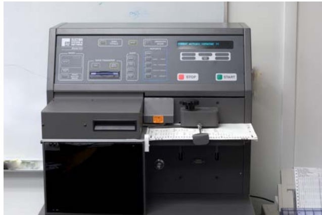
ES&S Model 650 Central Count Optical Scanner
