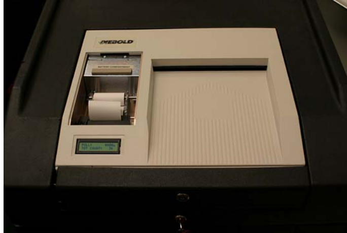
Premier's AccuVote Optical Scanner (AV-OS)
