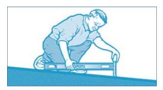
Image 9.3: Measuring slope using a 24-inch level and tape measure.
