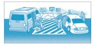
Image 9.6: Van-accessible parking spaces serve both cars and vans. A wide access aisle is needed so a wheelchair lift may be lowered from the van onto the level surface.
