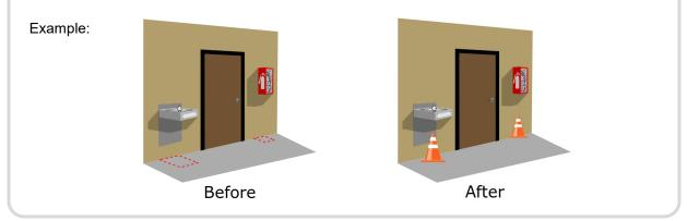
Image 3: The instructions above explain how to make a protruding object cane detectable.
