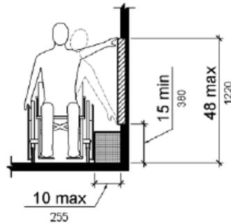
Unobstructed side reach with an allowable obstruction less than 10 inches (254 mm) deep.
