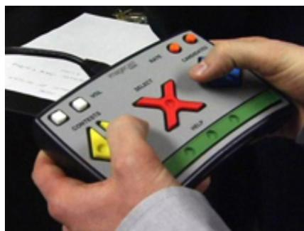
**Ballot Marking Devices and Systems** provide an interface to assist voters with disabilities in marking a paper ballot, which is then scanned or counted manually. Most ballot marking devices provide a touchscreen interface together with audio and other accessibility features similar to those provided with DREs, but rather than recording the vote directly into computer memory, the voter's selections are indicated through a marking a paper ballot, which is then scanned or counted manually.
