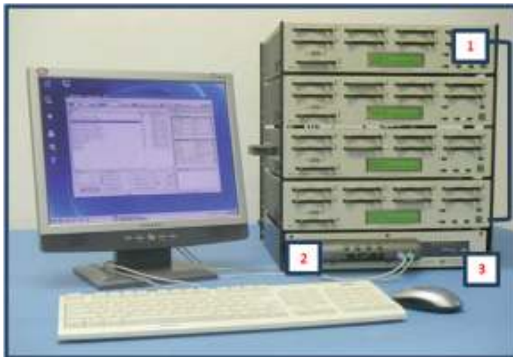
Figure 121: Typical Duplicator KVM Switch Setup
