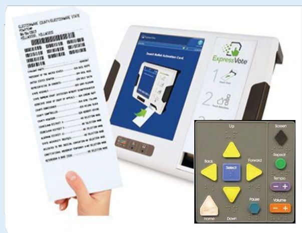
The picture above depicts the ExpressVote voting machine, ballot and tactile pad (with Braille).
