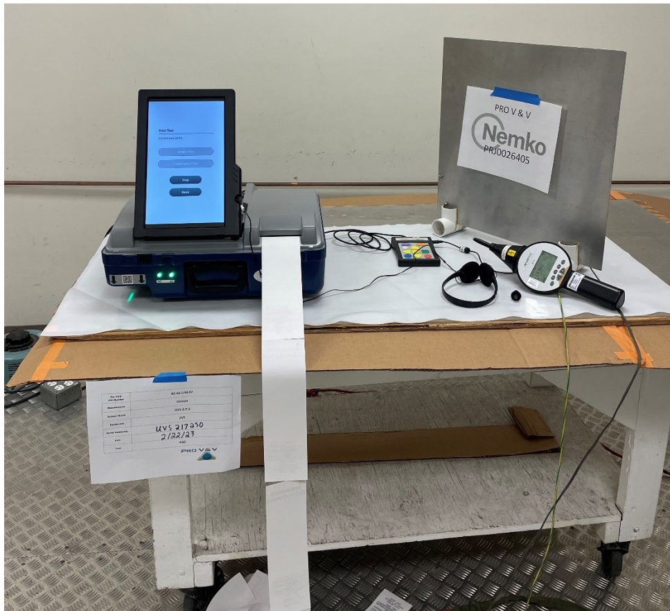
Figure 3.1-7: Electrostatic discharge setup
