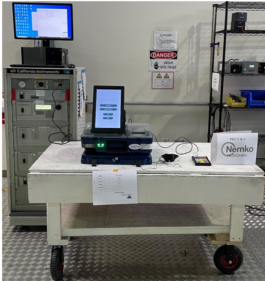
Figure 3.7-1: Voltage dips and voltage interruptions setup
