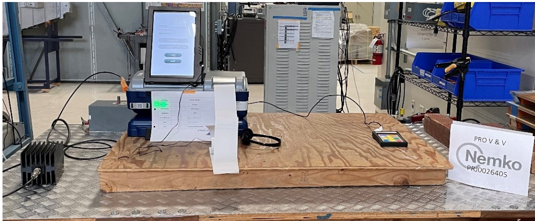
Figure 3.5-1: Continuous RF electromagnetic field disturbance setup
