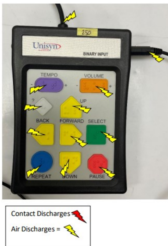
Figure 3.1-4: Electrostatic discharge test points
