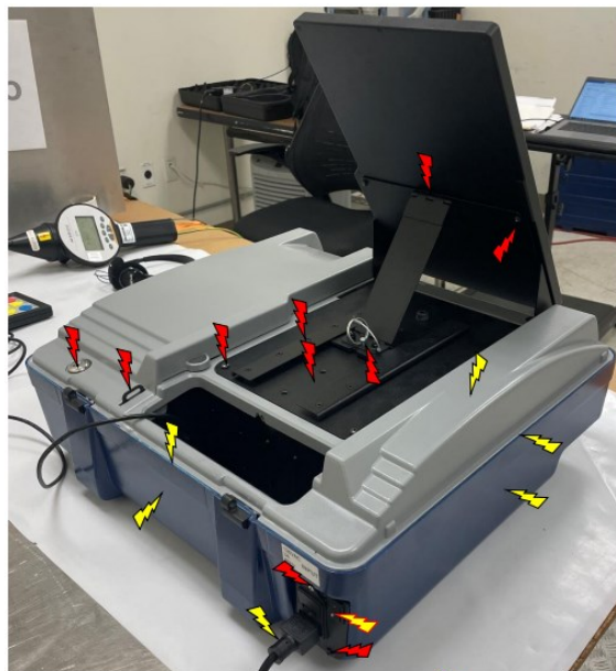
Figure 3.1-2: Electrostatic discharge test points
