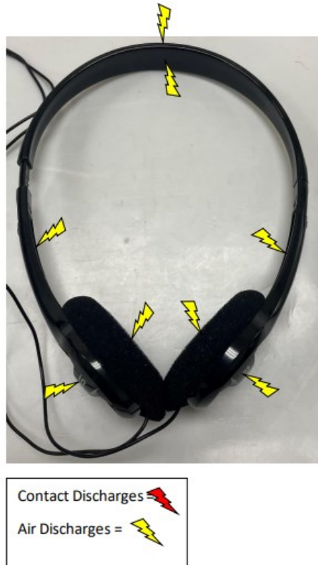
Figure 3.1-6: Electrostatic discharge test points
