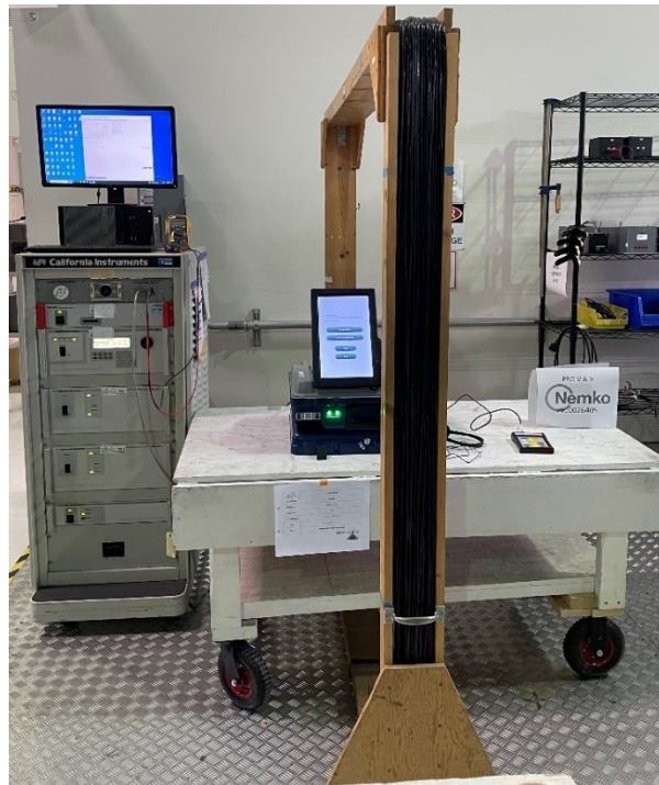
Figure 3.6-1: Power frequency magnetic field setup
