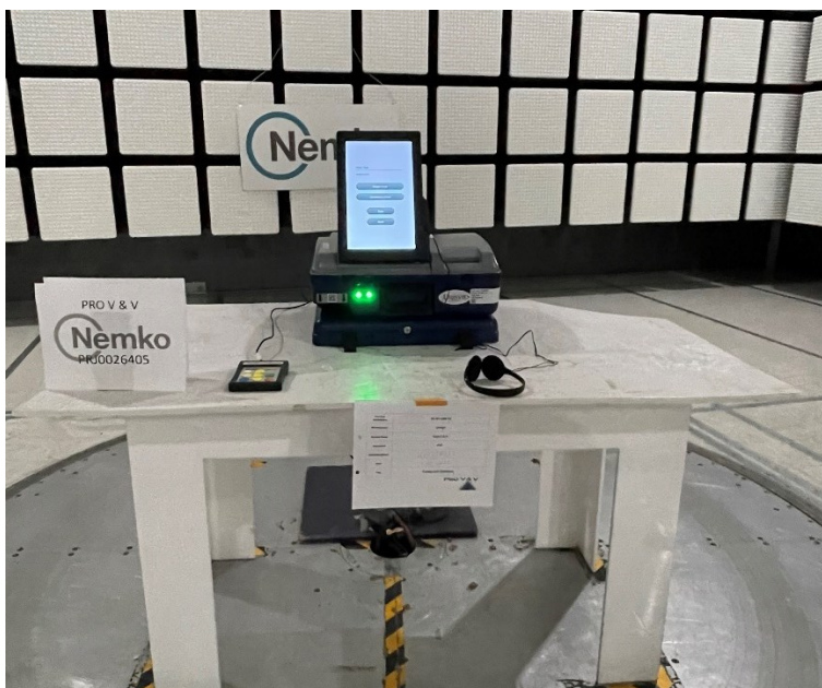
Figure 2.1-2: Radiated emissions setup photo below 1 GHz
