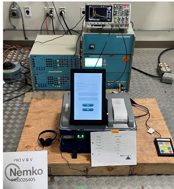
Figure 3.3-1: Electrical fast transients / burst setup (AC mains)
