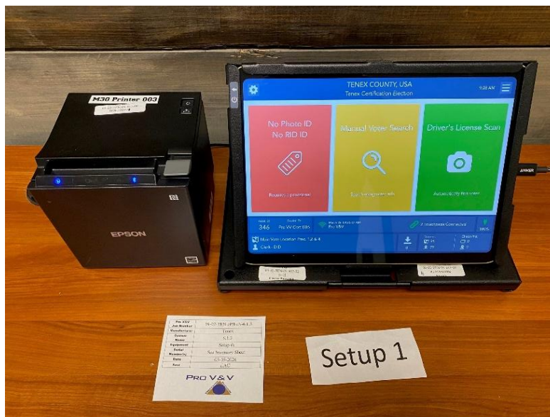
Photograph 1: Precinct Central 6.1.3 - Testing Setup 1 iPad 11th GEN (KT77J2L659N), Stand ([S-1]), Epson Printer ([TEN-100741])
