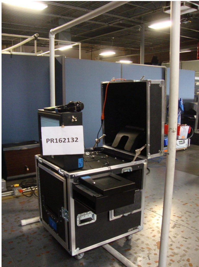
Power Frequency H-Field Immunity Setup
