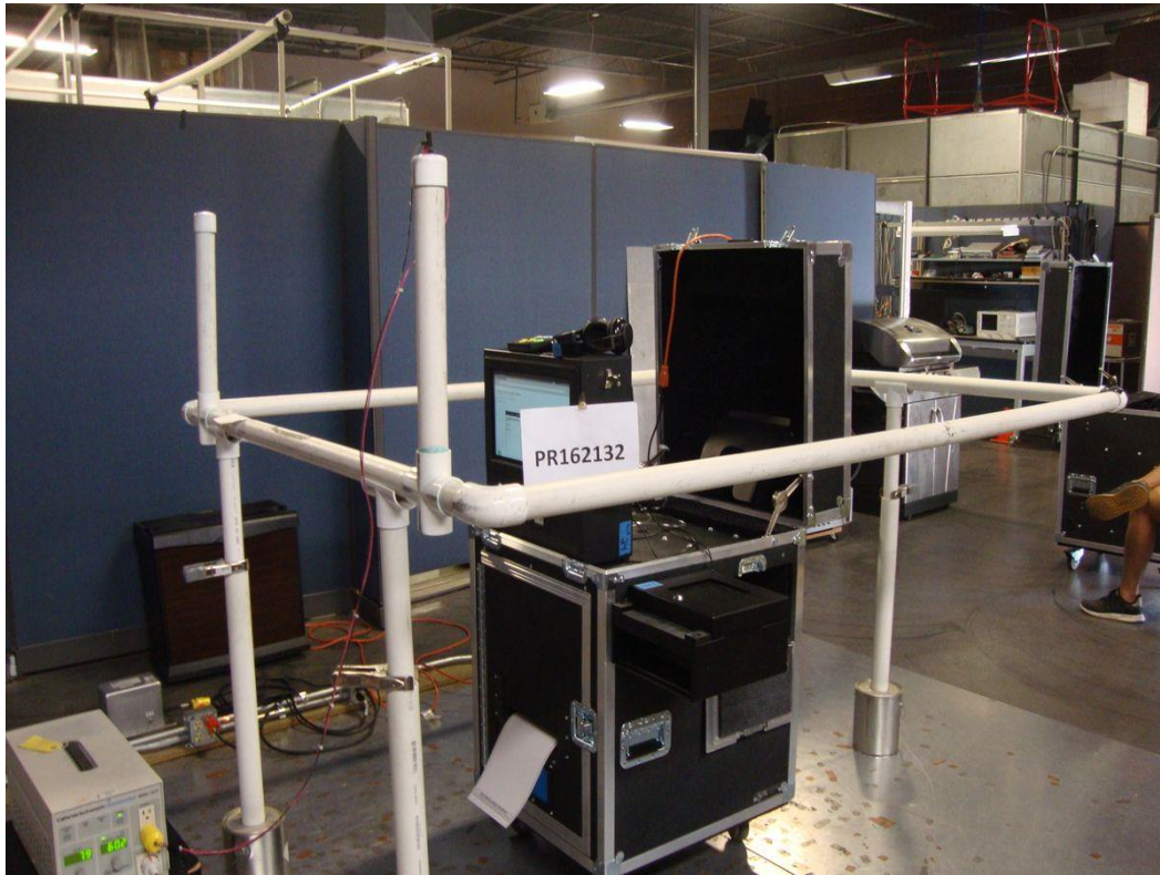
Power Frequency H-Field Immunity Setup
