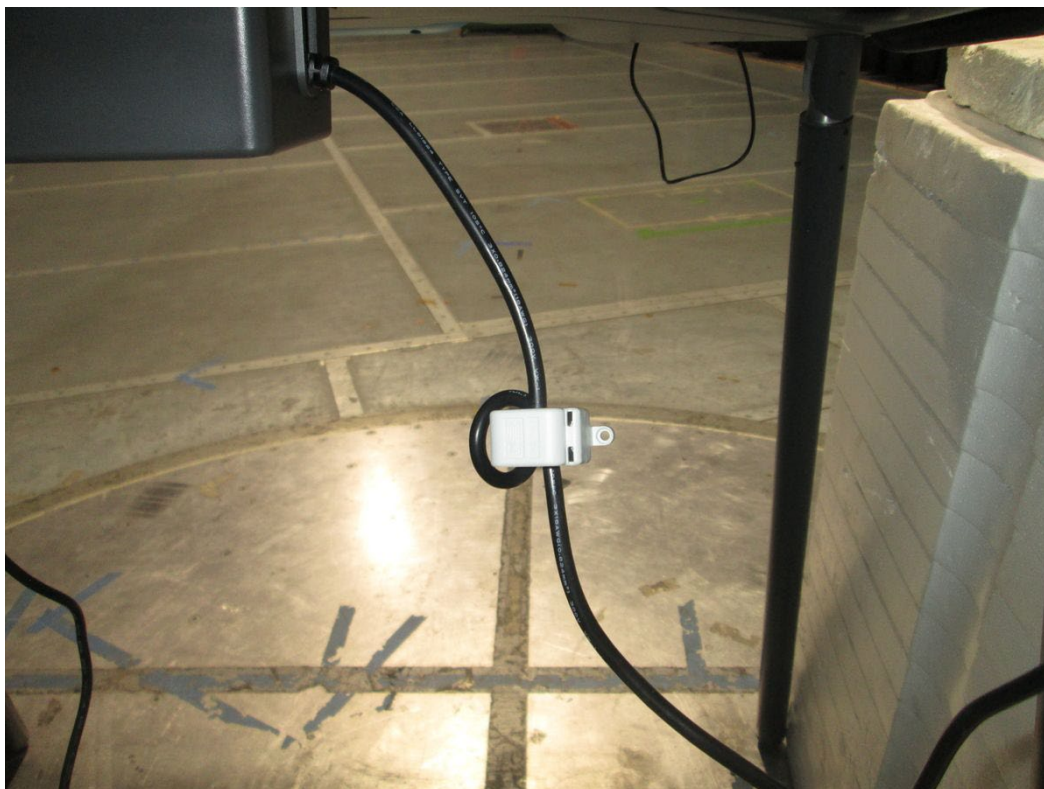
Radiated Emissions Ferrite Placement
