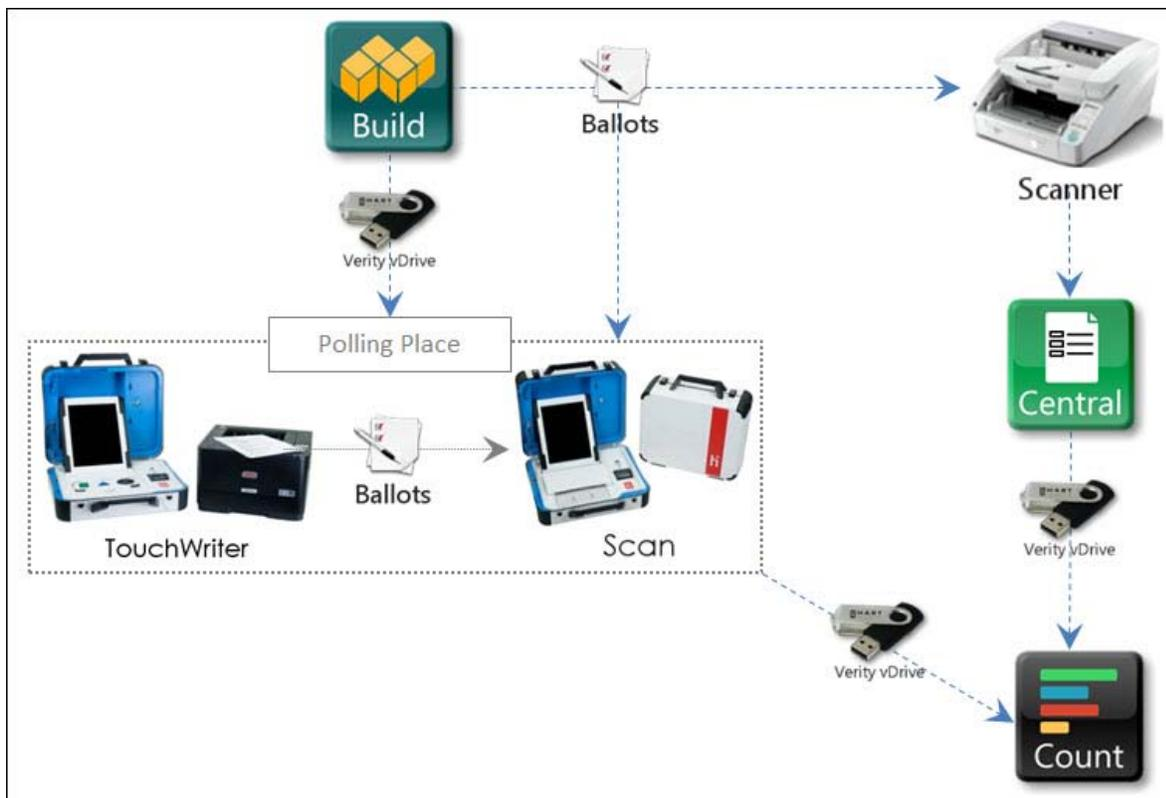
Figure 1 - Verity Voting System Diagram
