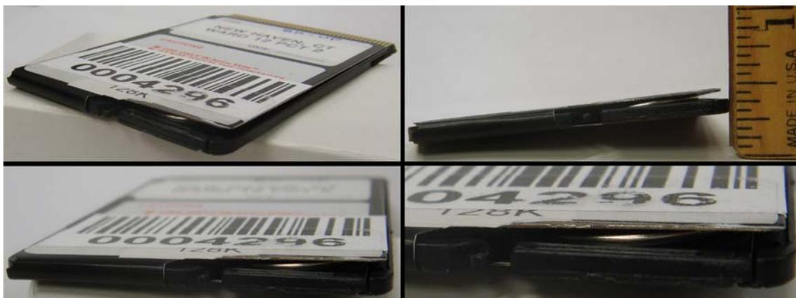
Figure 1: Memory Card – enclosure is apart from frame
