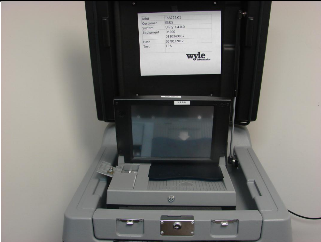
Photograph 1: ES&S Unity 3.4.0.0 FCA Test Setup
