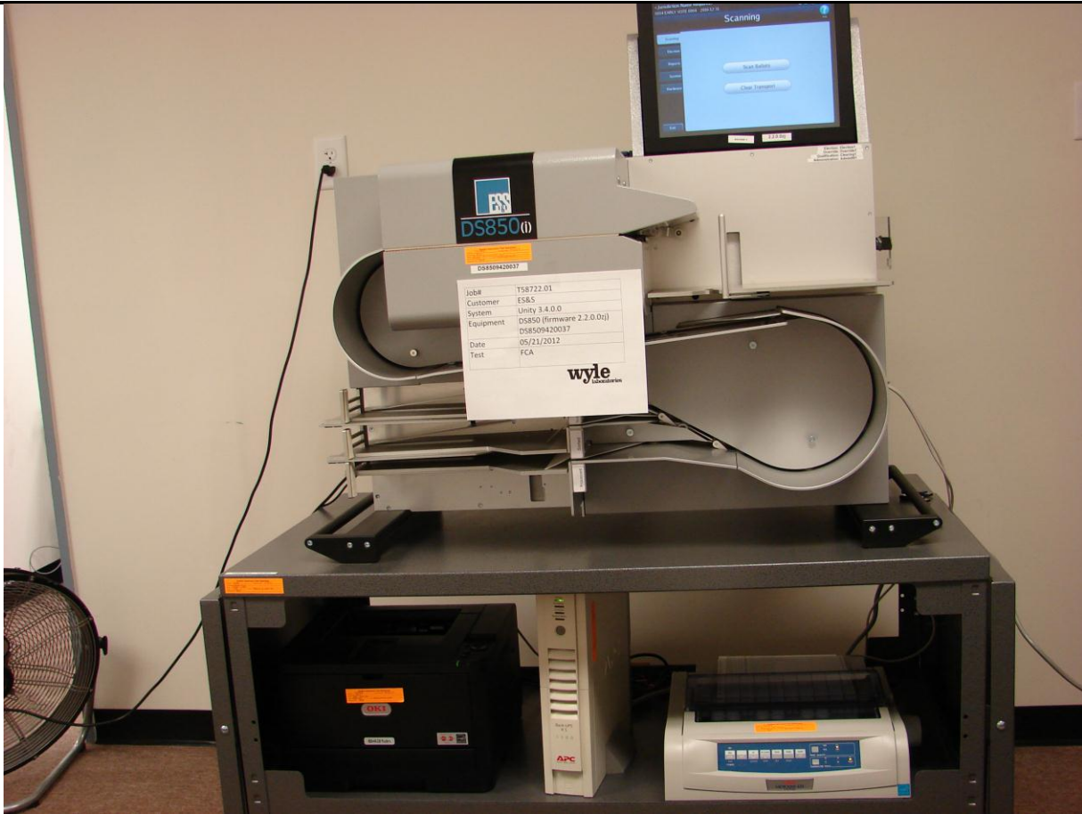
Photograph 2: ES&S Unity 3.4.0.0 FCA Test Setup
