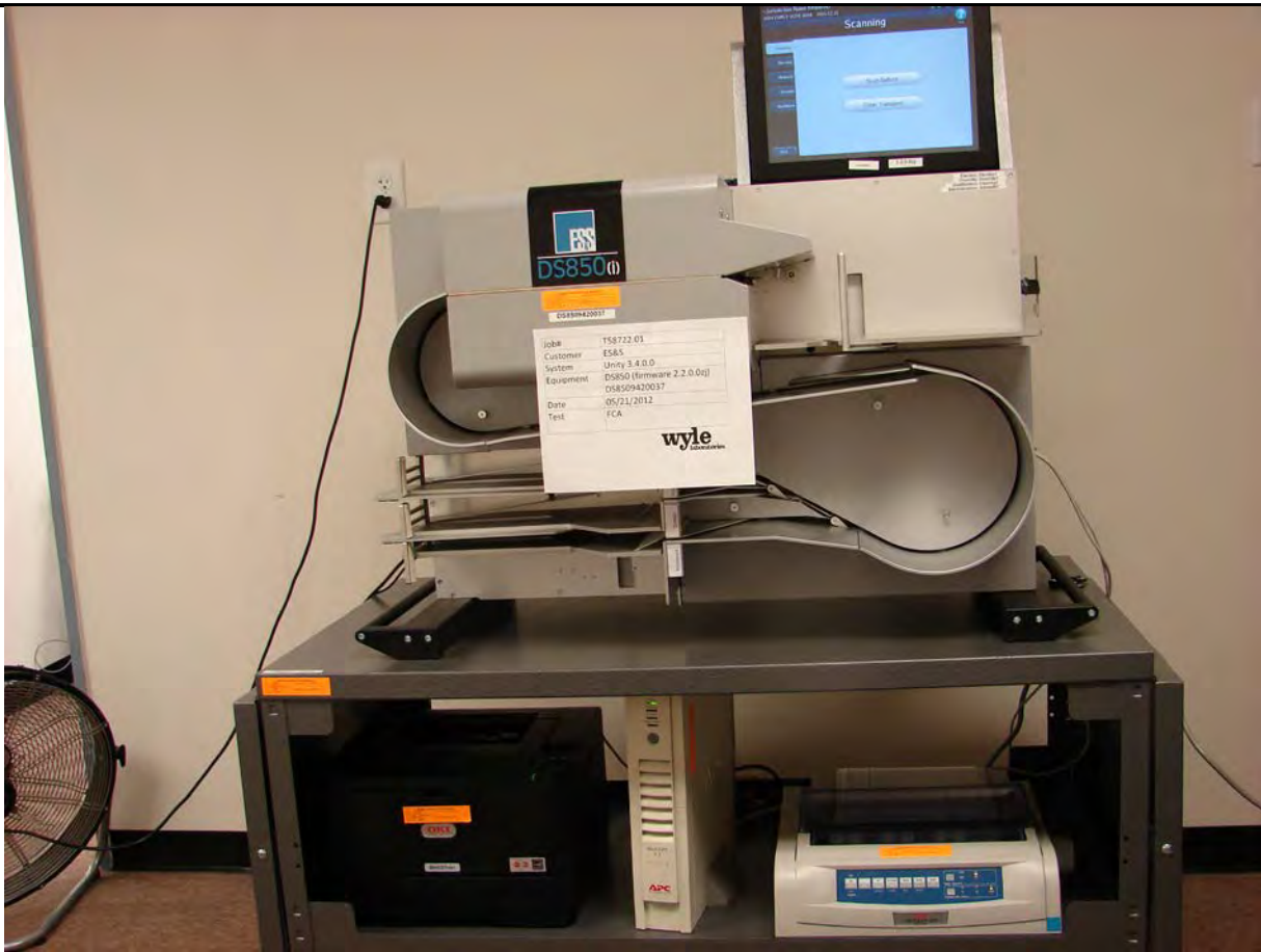
Photograph 2: ES&S Unity 3.4.0.0 FCA Test Setup
