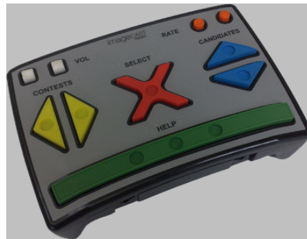
Figure 1.3: Audio Tactile Interface (ATI)
