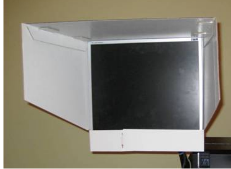
Figure 1.4: The adjustable arm-mounted LCD is shielded with a privacy cowl
