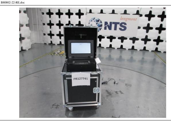
Figure A1: Radiated Emissions Test Setup – Front Side
