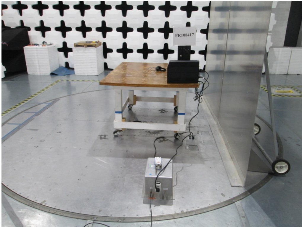
Figure B4: Conducted Emissions Test Setup – Right Side
