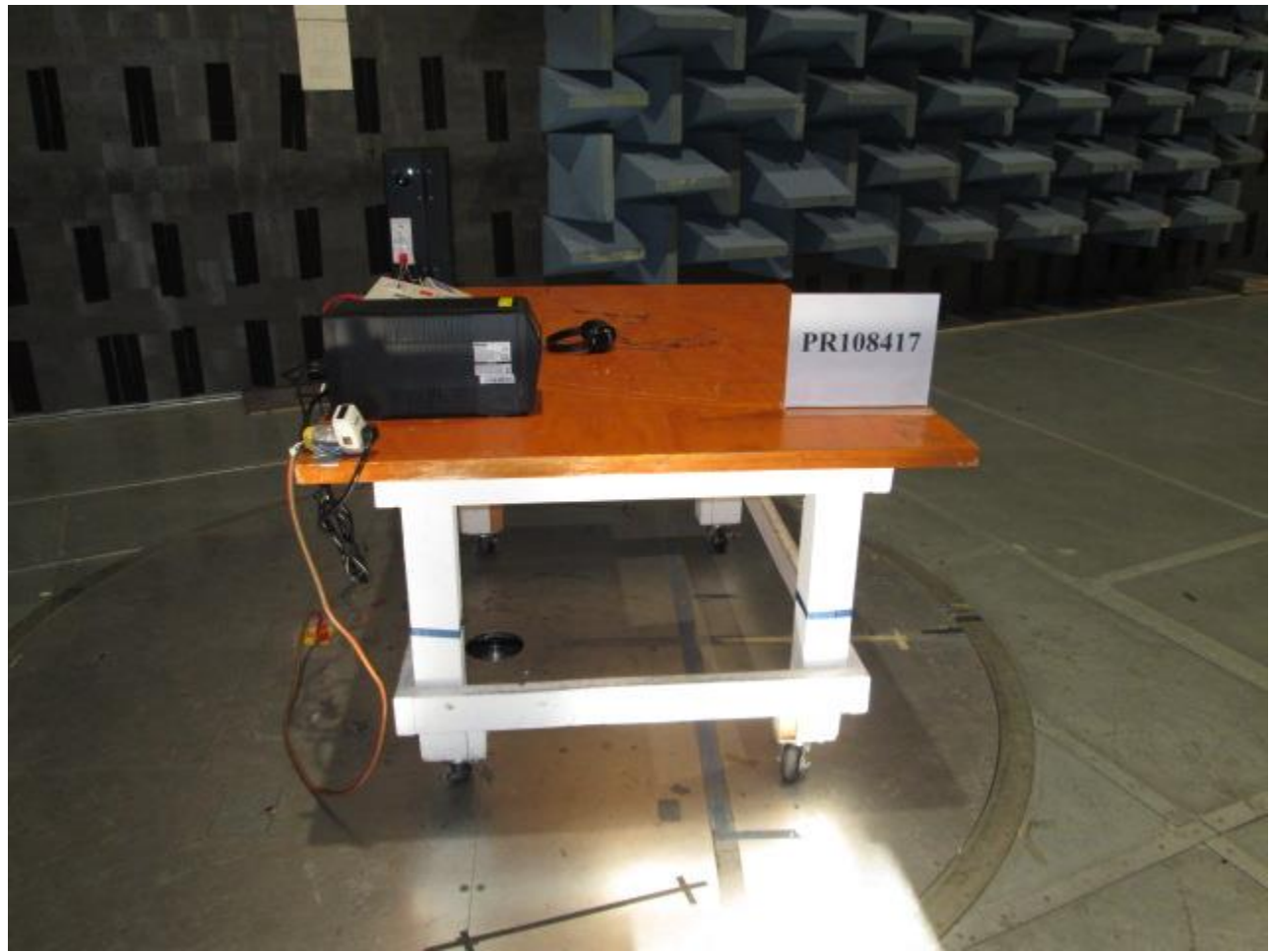
Figure A5: Radiated Emissions Test Setup – Left Side
