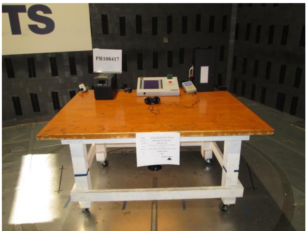
Figure A2: Radiated Emissions Test Setup – Front Side
