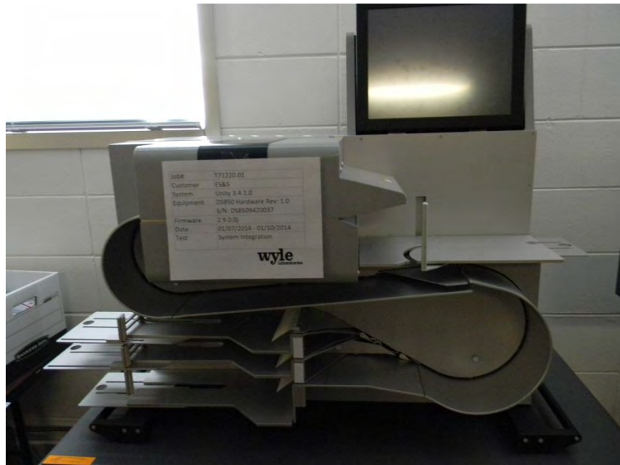
Photograph No. 10 DS850 System Integration Test Setup
