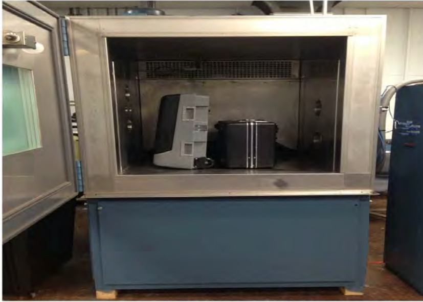
Photograph 29: ES&S FL EVS 4.5.0.0 Low Temperature
