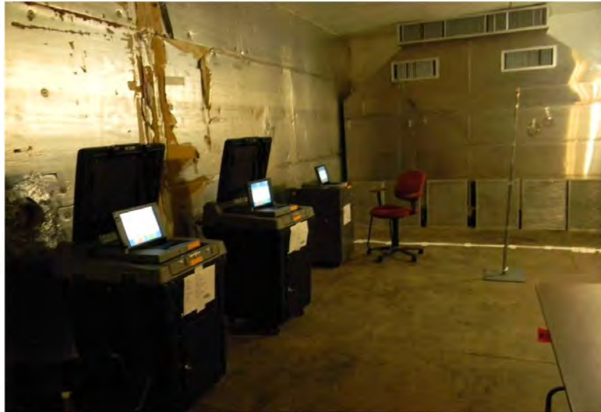
Photograph 24: ES&S FL EVS 4.5.0.0 Temperature and Power Variation
