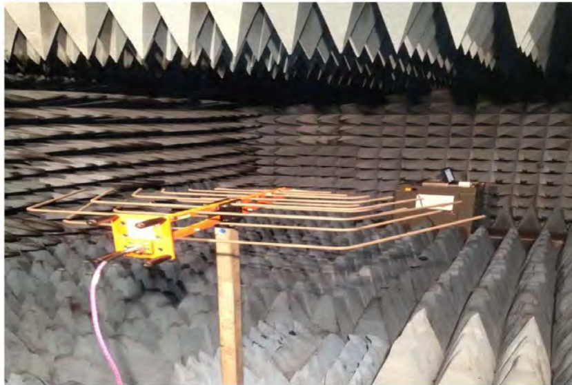
Photograph 21: ES&S FL EVS 4.5.0.0 Electromagnetic Susceptibility
