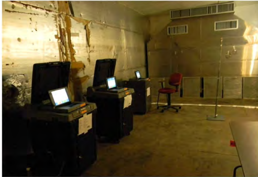
Photograph 24: ES&S FL EVS 4.5.0.0 Temperature and Power Variation
