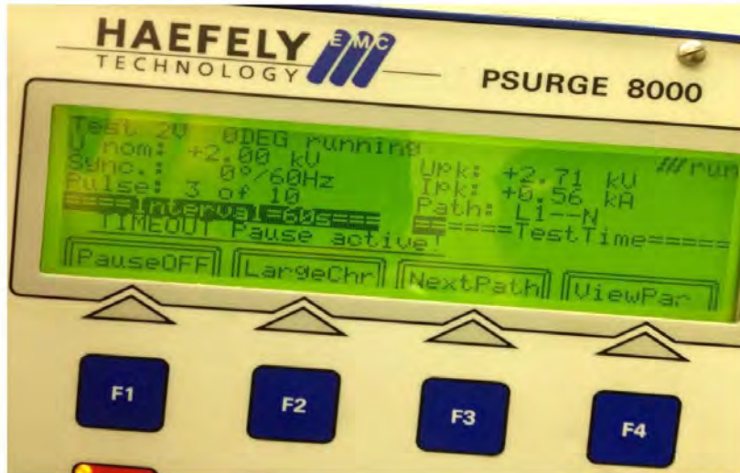
Photograph 11: ES&S FL EVS 4.5.0.0 Lightning Surge
