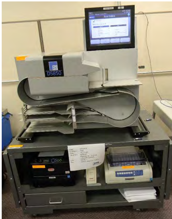
Photograph No. 15 DS850 System Integration Test Setup
