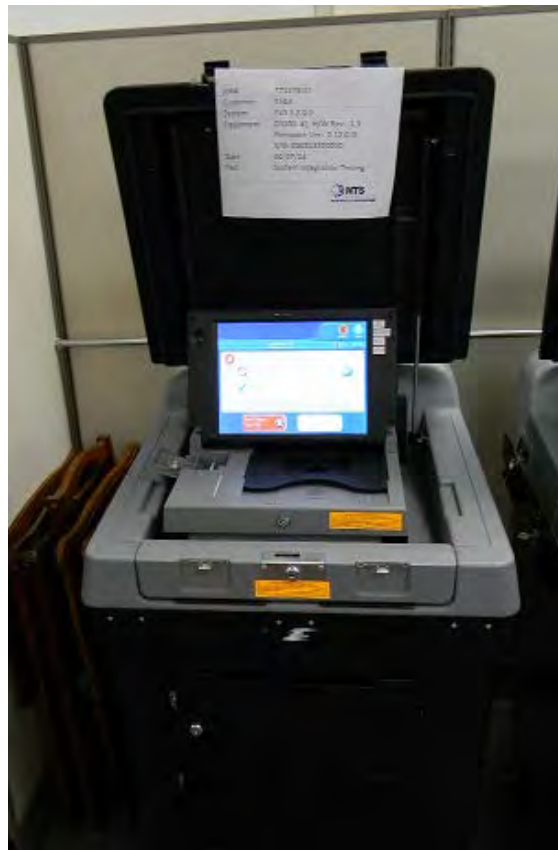
Photograph No. 12 DS200 System Integration Test Setup
