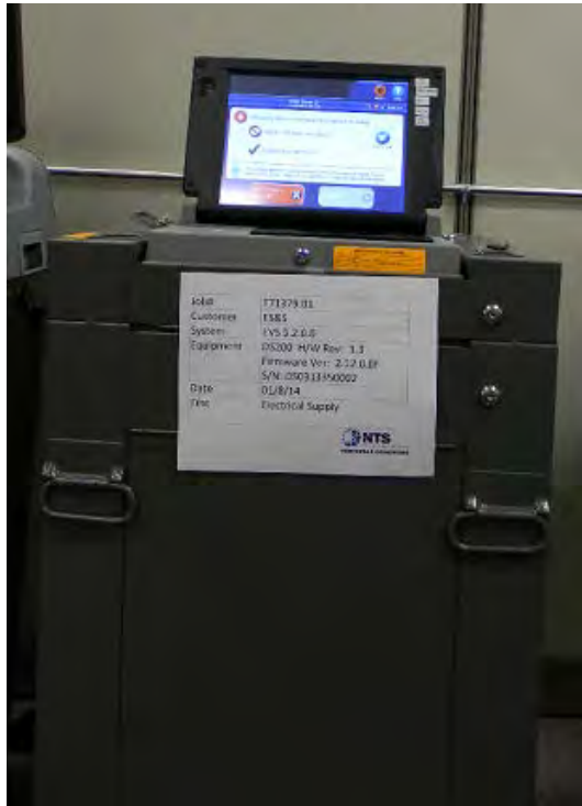
Photograph No. 2 DS200 Electrical Supply Test Setup
