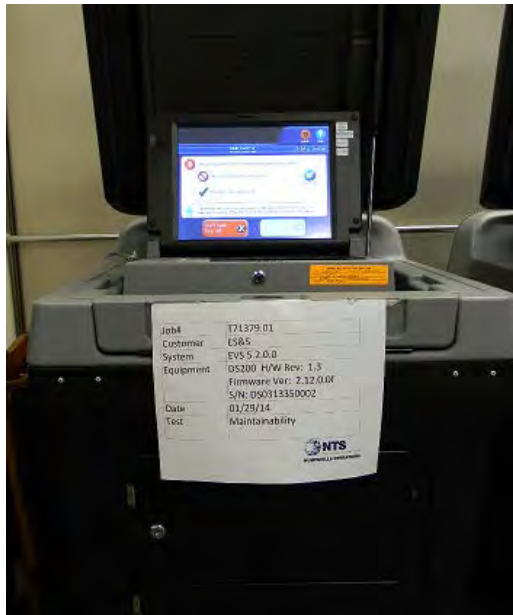
Photograph No. 4 DS200 Maintainability Test Setup
