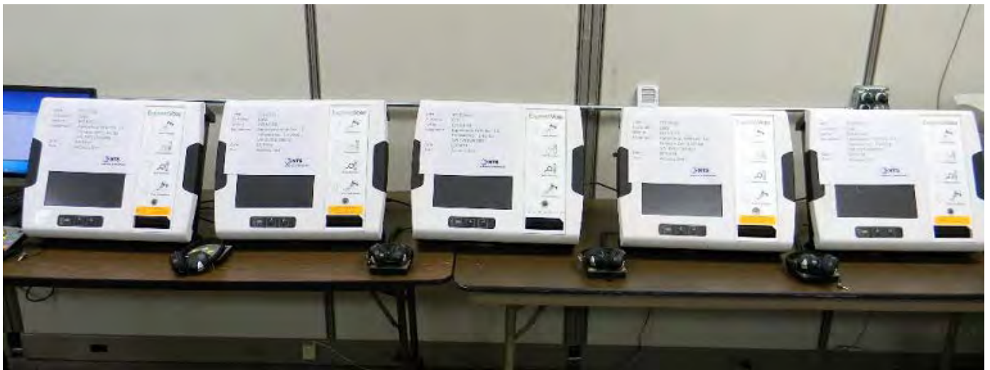
Photograph No. 8 ExpressVote Accuracy Test Setup
