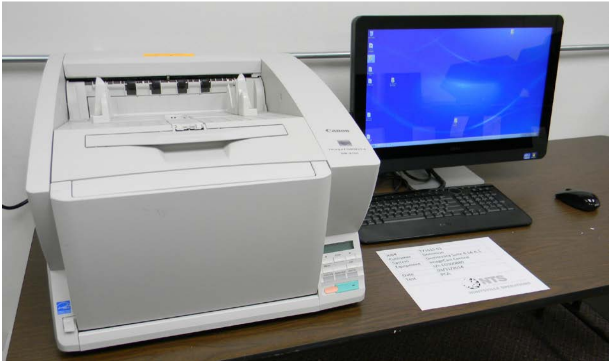
Figure No. 3 Canon DR-X10C Scanner and ImageCast Central Workstation
