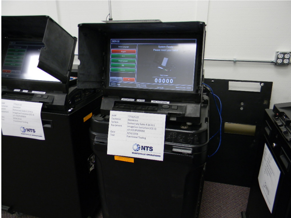
Photograph 4 Functional Testing: ImageCast Evolution
