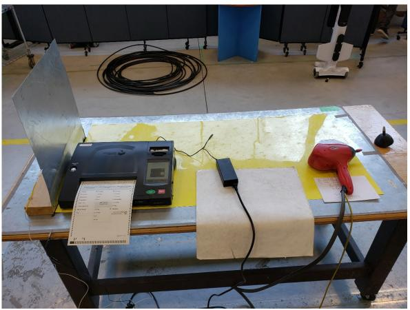
Figure 13 – Electrostatic Disruption Setup
