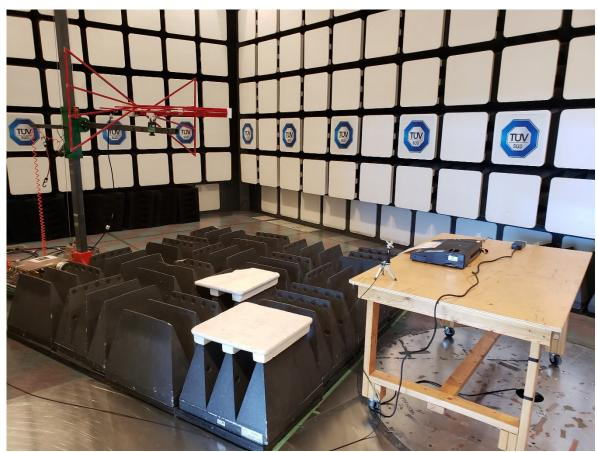
Figure 15 – Electromagnetic Susceptibility Setup – Photo 2
