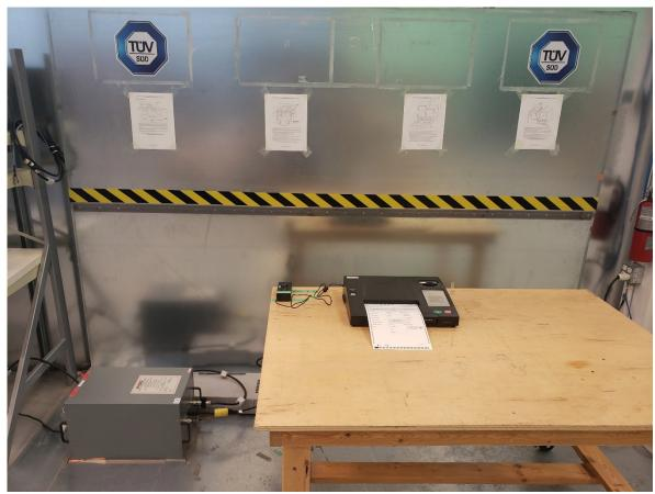
Figure 5 – Power Line Conducted Emissions Setup – Photo 1
