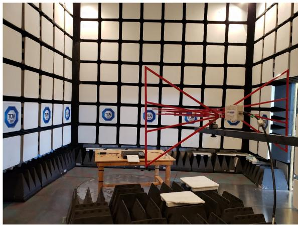
Figure 14 – Electromagnetic Susceptibility Setup – Photo 1
