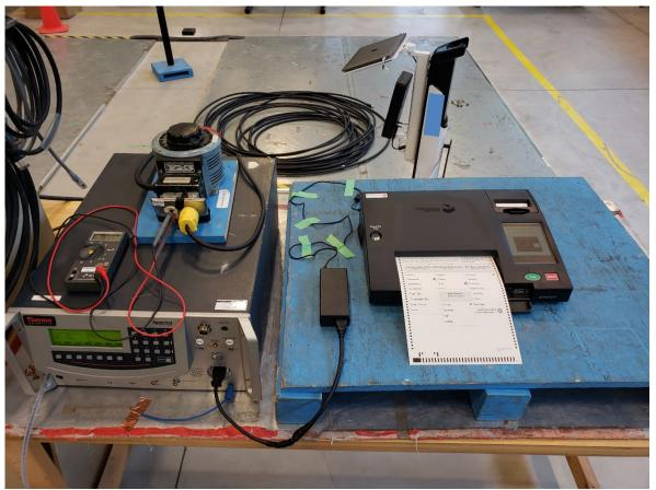
Figure 9 – Electrical Power Disturbance – Surges of ±15% Line Variations
