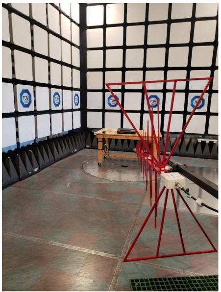
Figure 7 – Radiated Emissions Setup – Photo 1 30MHz – 1GHz
