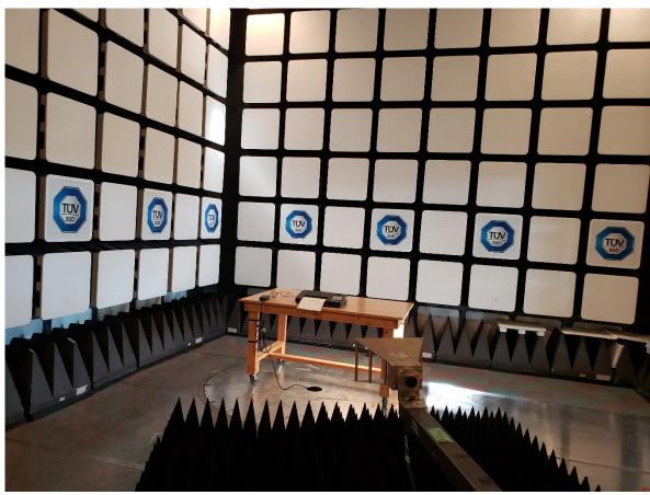
Figure 8 – Radiated Emissions Setup – Photo 2 1GHz – 6GHz
