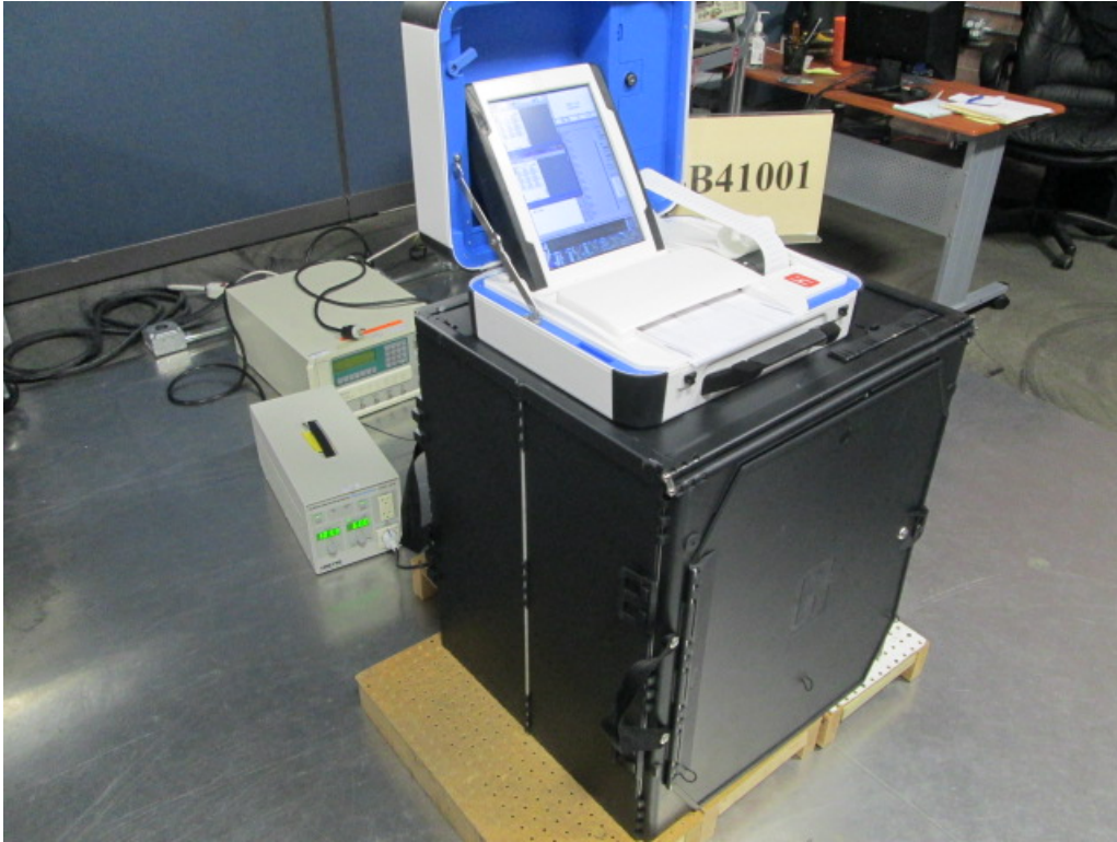
Figure G3. Voltage Dips and Interrupts Test Setup. +/-15% voltage variations
