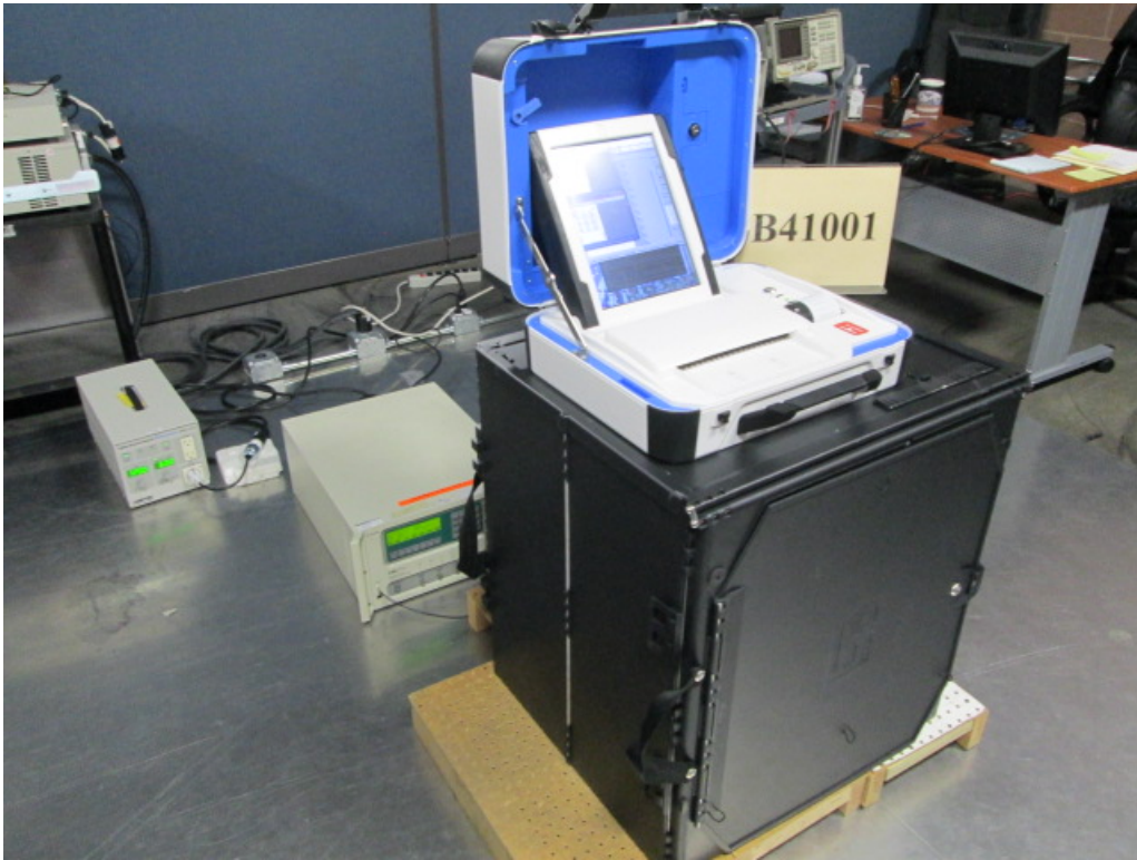
Figure D1. Surge Immunity Test Setup
