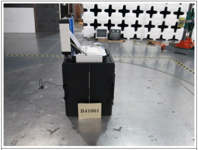
Figure A6: Radiated Emissions Test Setup – Left Side
