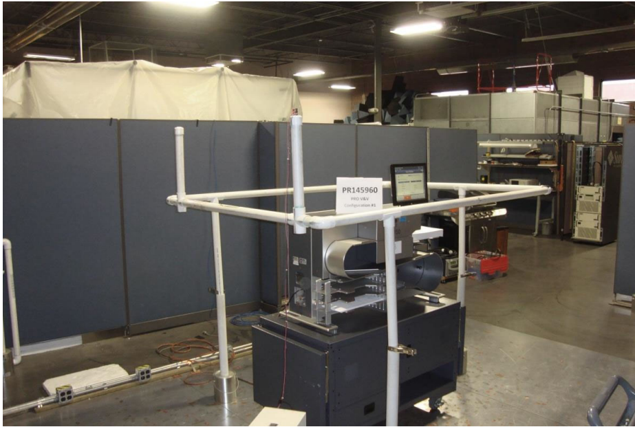
Power Frequency H-field Immunity Test Setup (Config #1)
