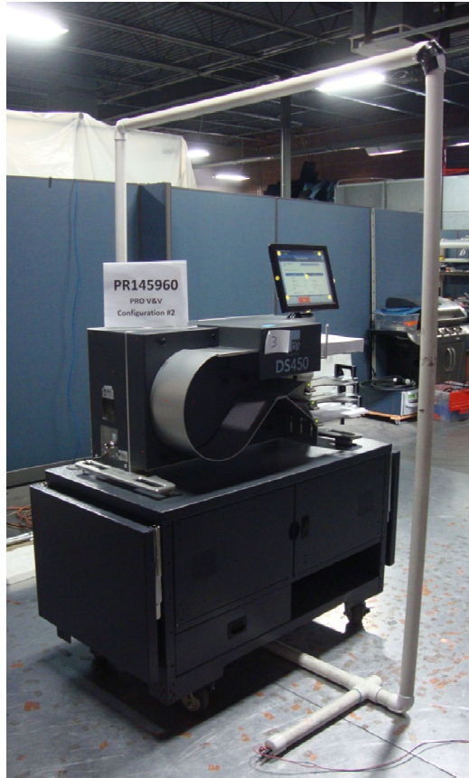
Power Frequency H-field Immunity Test Setup (Config #2)
