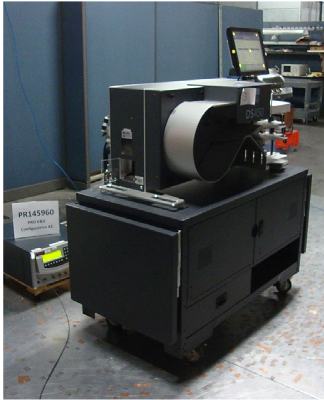
Electrical Fast Transient Test Setup (Config #2)
