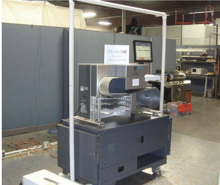
Power Frequency H-field Immunity Test Setup (Config #1)
