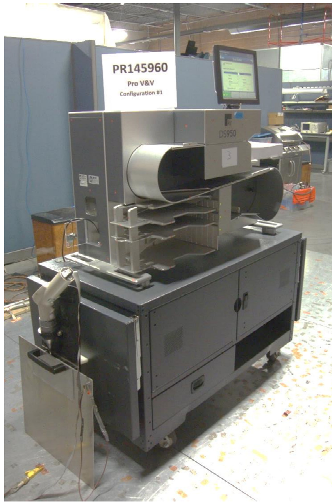
Figure 1: Electrostatic Discharge Test Setup (Config #1)
