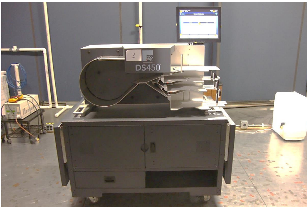
Figure 2. Electrostatic Discharge Test Setup (Config #2)
