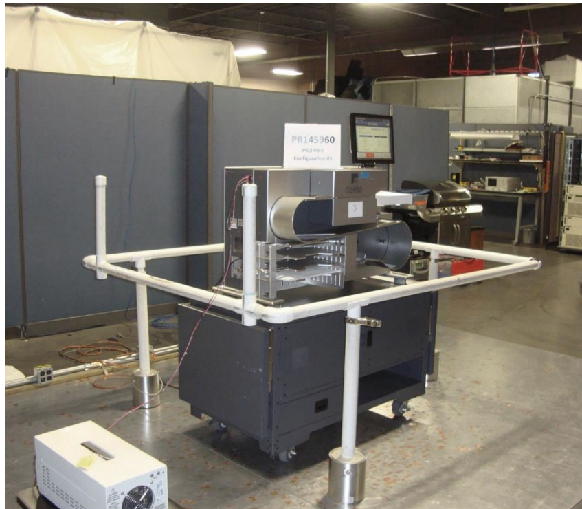
Power Frequency H-field Immunity Test Setup (Config #1)
