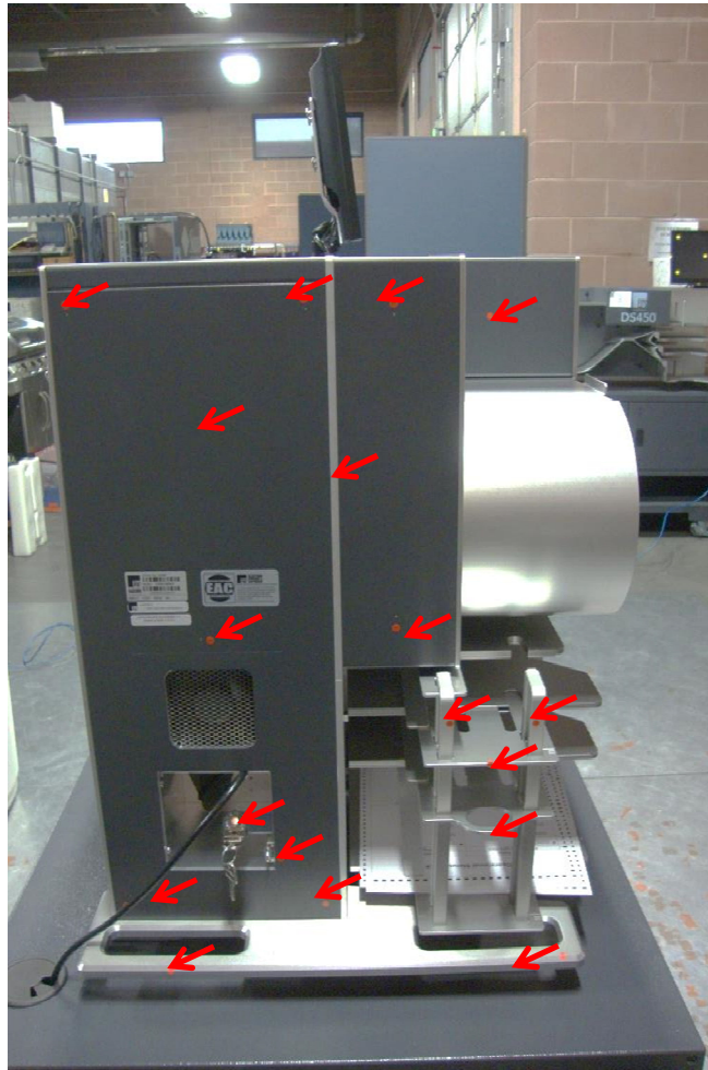
Figure 6. Electrostatic Discharge Test Points
