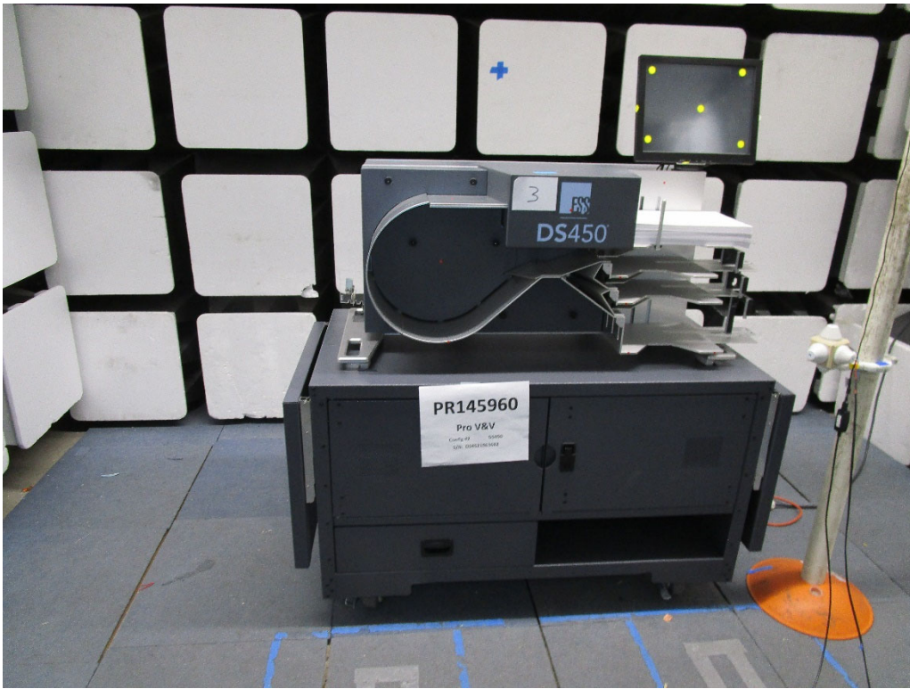
Radiated RF Immunity Test Setup – Front Side (Config #2)
