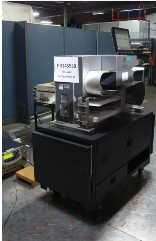
Voltage Dips and Interruptions Test Setup (Config #1)
