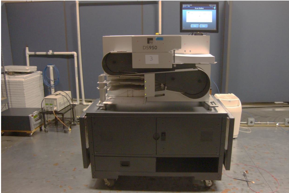
Figure 2. Electrostatic Discharge Test Setup (Config #1)
