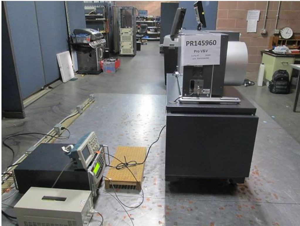
Voltage Dips and Interruptions Test Setup (Config #2)
