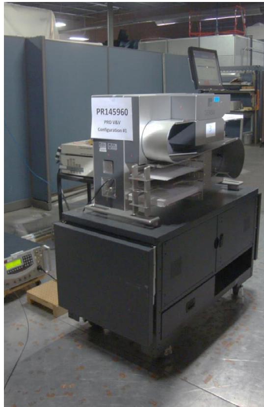
Surge Immunity Test Setup – AC Mains (Config #1)
