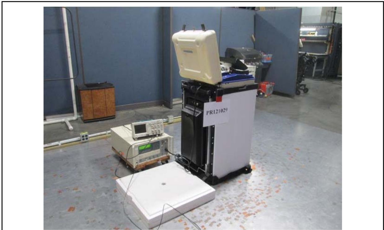
Figure C1. Electrical Fast Transient Test Setup.
