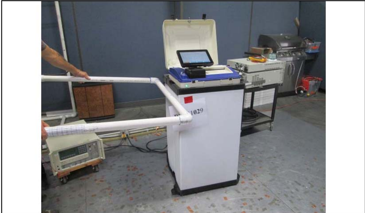
Figure F2. Power Frequency H-field Immunity Test Setup.
