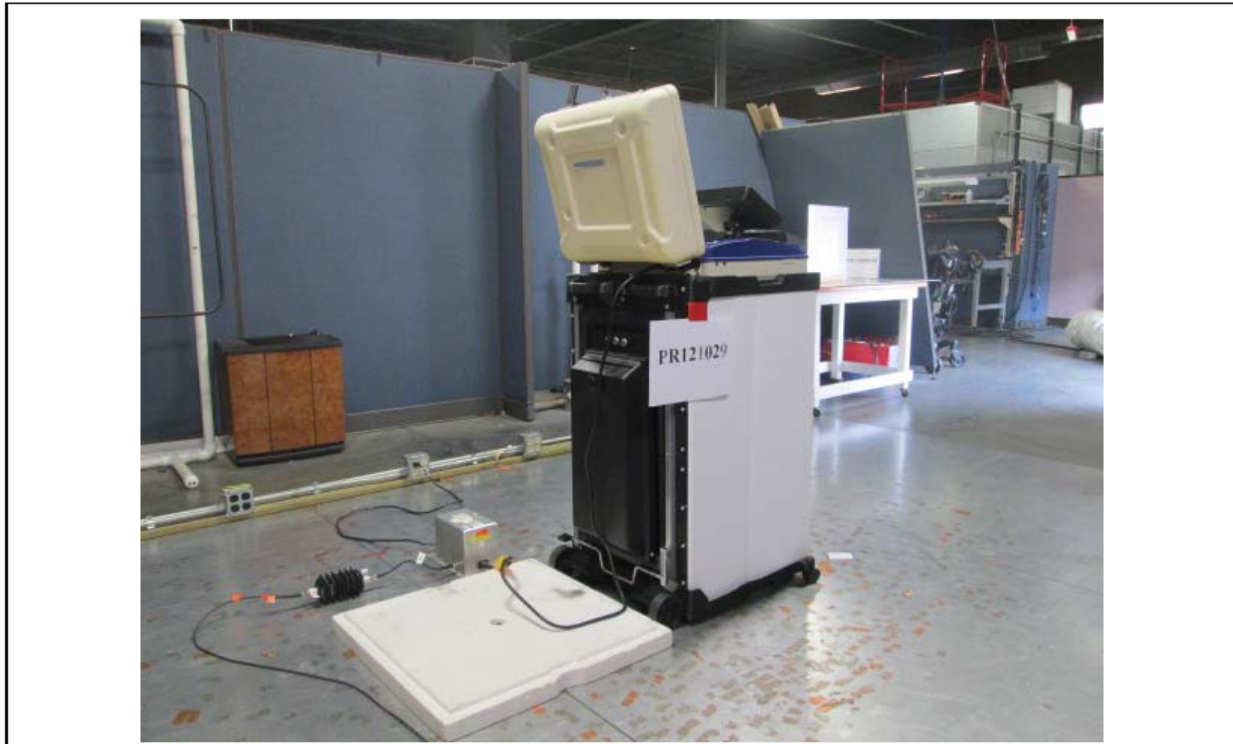
Figure E1. Conducted RF Immunity Test Setup.
