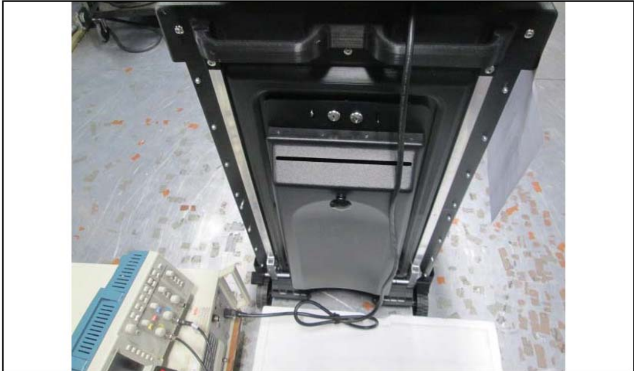
Figure C2. Electrical Fast Transient Test Setup – AC Mains.
