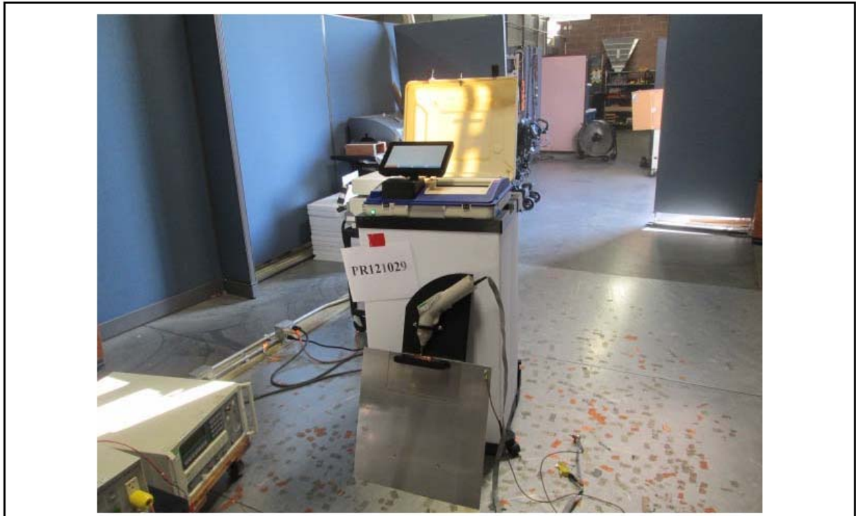
Figure A1. Electrostatic Discharge Test Setup.
