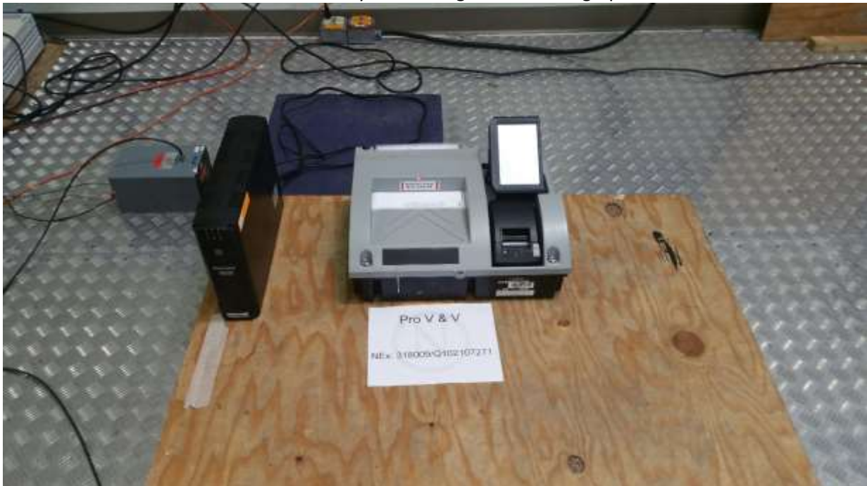
Conducted RF Immunity Test Configuration Photograph - OVO
