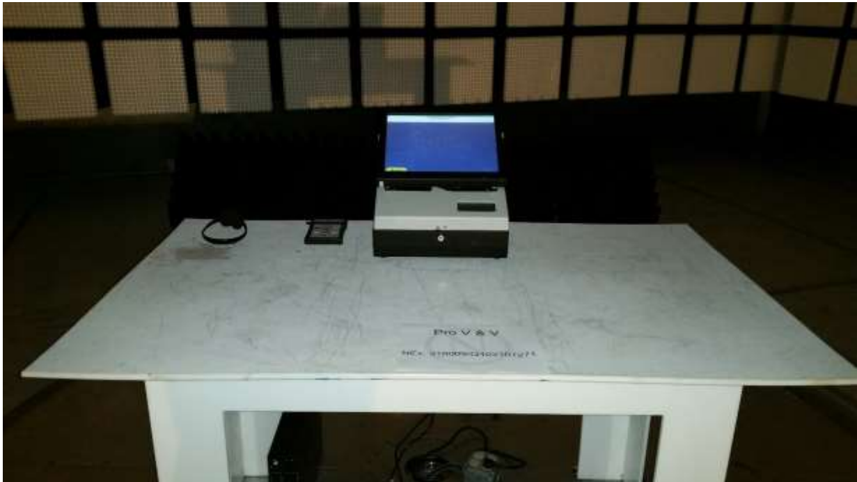
Radiated Emissions Test Configuration Photograph - Above 1GHz - OVI-VC
