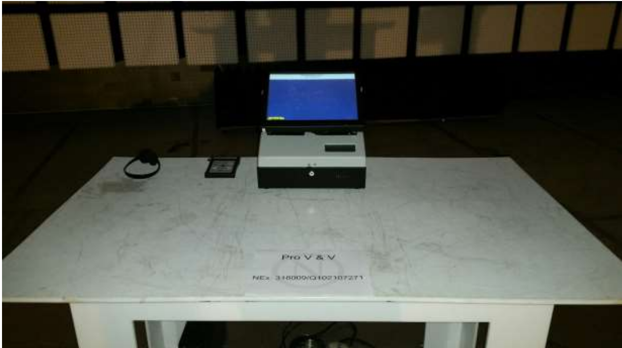
Radiated Emissions Test Configuration Photograph - Below 1GHz - OVI-VC
