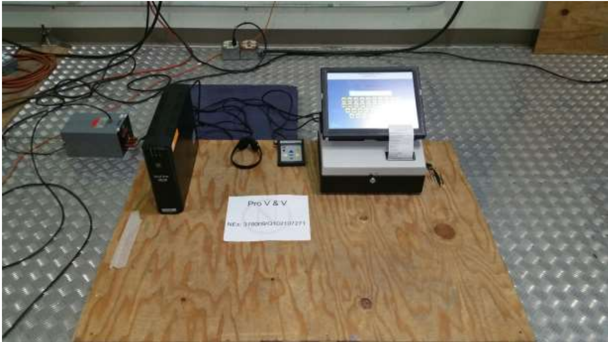
Conducted RF Immunity Test Configuration Photograph - OVI-VC
