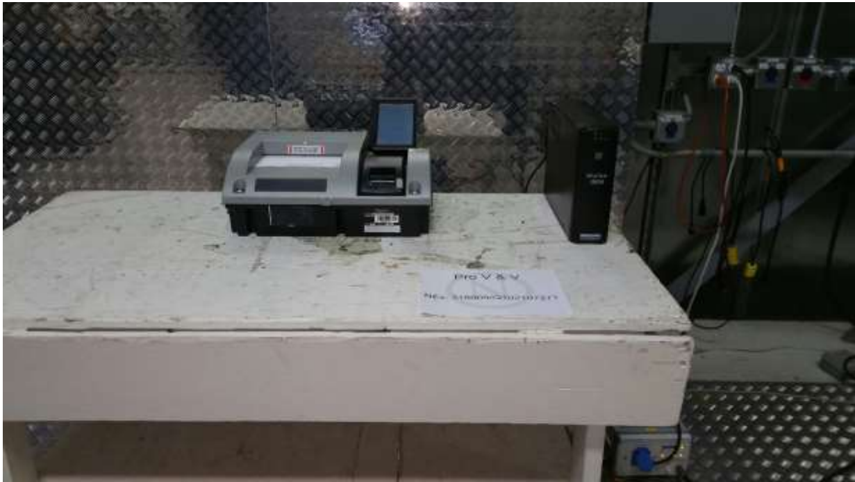
Conducted Emissions Test Configuration Photograph - OVO
