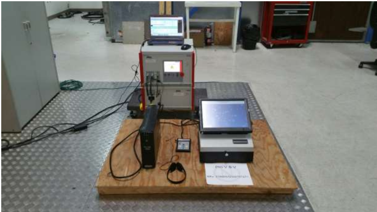
Lighting Surge Test Configuration Photograph - OVI-VC
