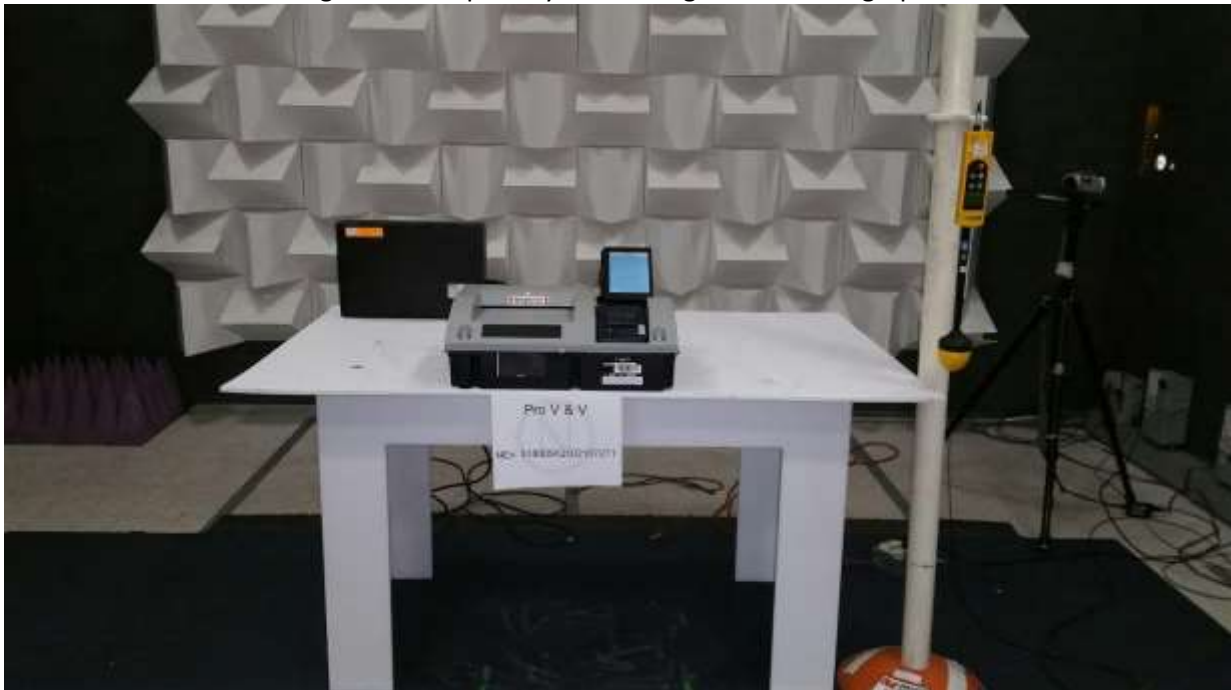
Electromagnetic Susceptibility Test Configuration Photograph - OVO
