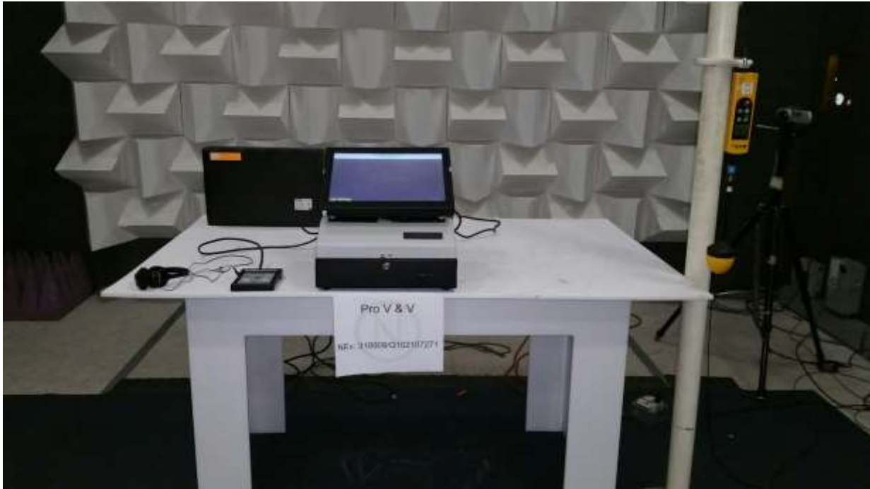
Electromagnetic Susceptibility Test Configuration Photograph - OVI-VC
