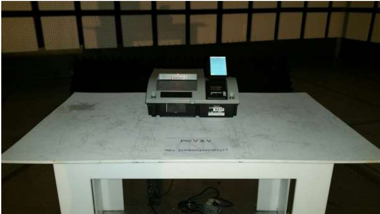
Radiated Emissions Test Configuration Photograph - Above 1GHz - OVO
