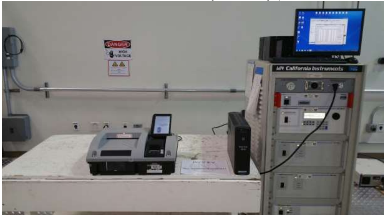
Electrical Power Disturbance Test Configuration Photograph - OVO
