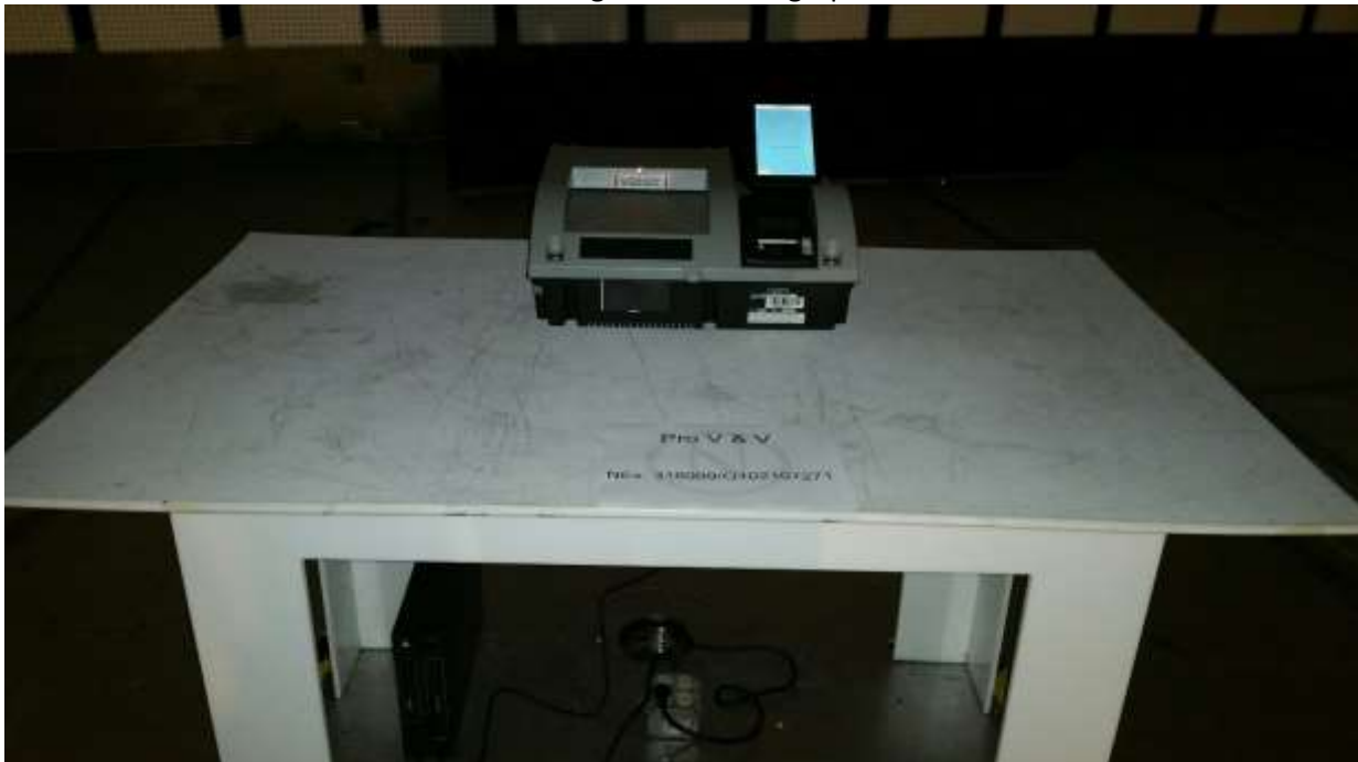
Radiated Emissions Test Configuration Photograph - Below 1GHz - OVO
