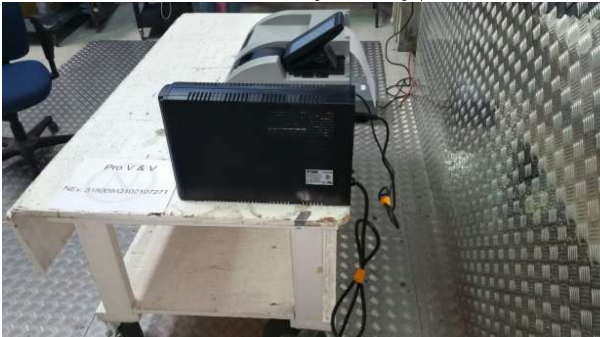
Conducted Emissions Test Configuration Photograph - OVO
