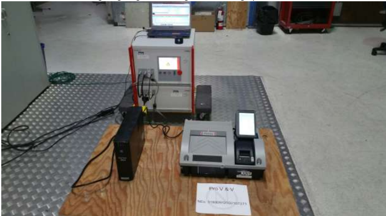
Lighting Surge Test Configuration Photograph - OVO
