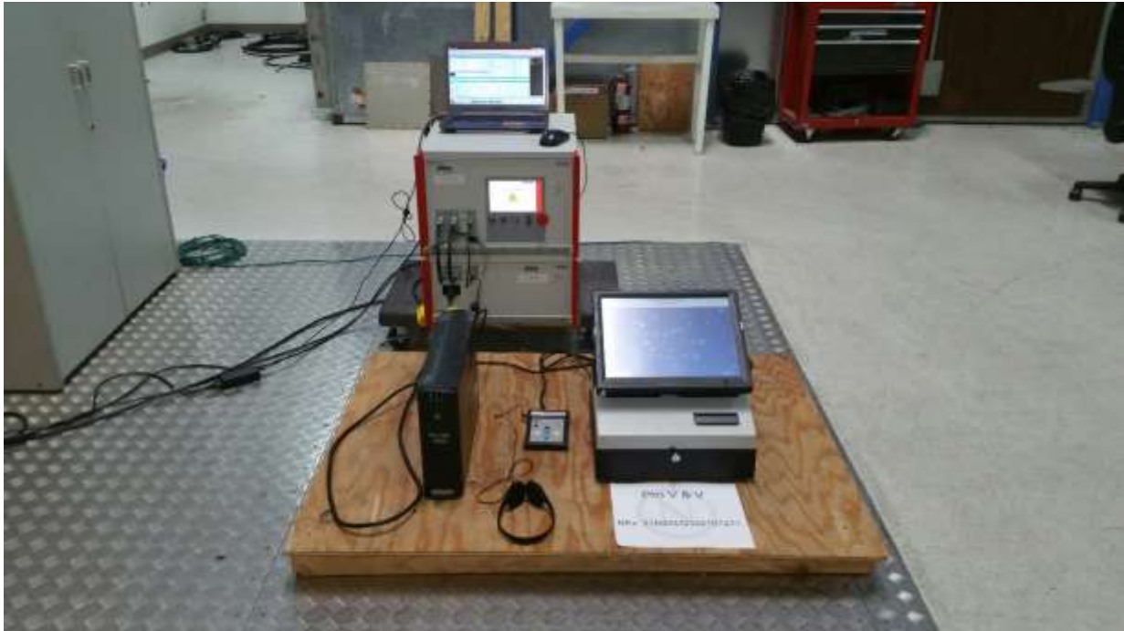
Lighting Surge Test Configuration Photograph - OVI-VC
