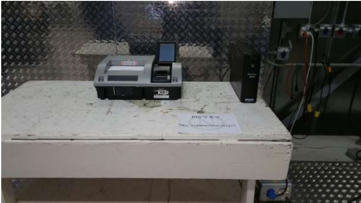
Conducted Emissions Test Configuration Photograph - OVO
