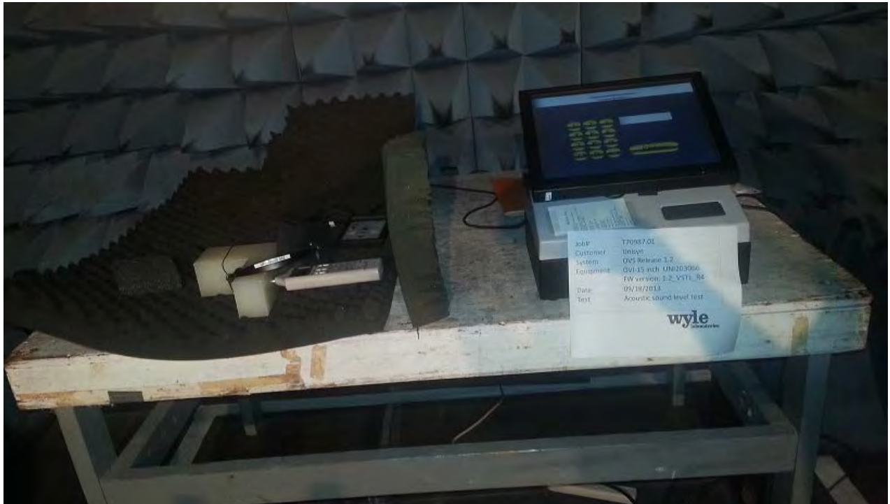
Photograph 11 Acoustic Sound Level Test Set Up
