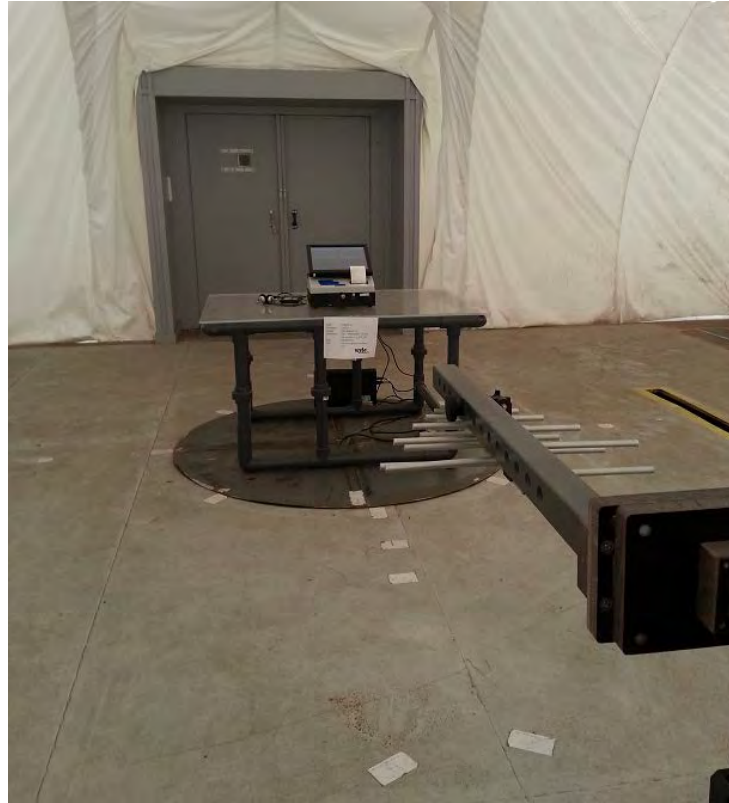
Photograph 8 Electromagnetic Radiation Test Set Up
