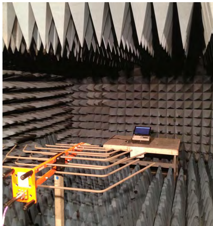
Photograph 9 Electromagnetic Susceptibility Test Set Up
