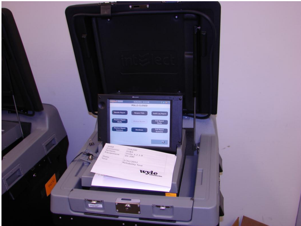
Photograph 4: ES&S Unity 3.2.1.0 Reliability Test Setup
