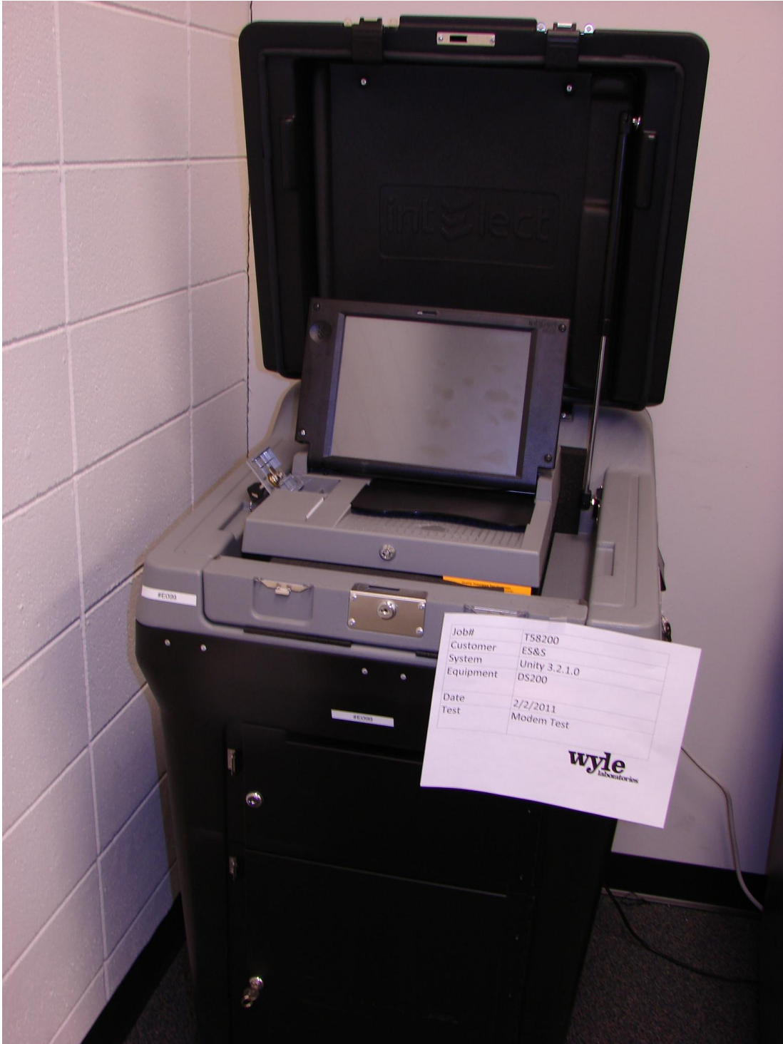
Photograph 5: ES&S Unity 3.2.1.0 Modem Test Setup
