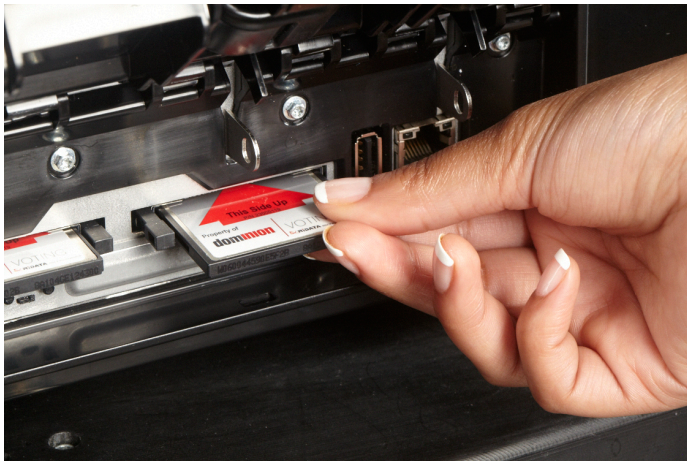
Figure 3.1: Inserting Compact Flash Cards
