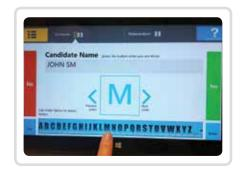
The EZ Ballot, a winning concept in the OpenIDEO challenge was developed in a graduate-level design class at the Georgia Institute of Technology. The final design combines tactile buttons, audio prompts, touch screen interaction and a slider for text entry.
