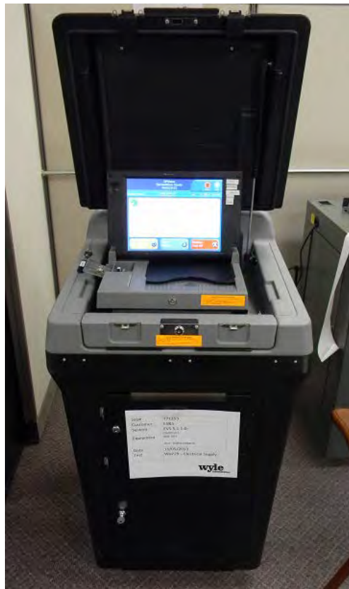
Photograph No. 8 ES&S EVS 5.0.1.0 Electrical Supply Test
