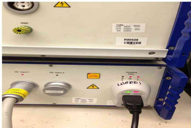
Photograph 12: ES&S FL EVS 4.5.0.0 Lightning Surge
