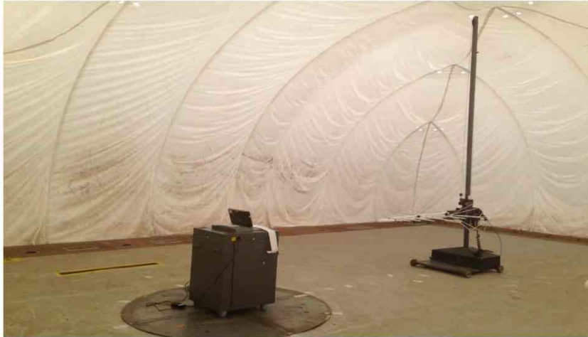
Photograph 15: ES&S FL EVS 4.5.0.0 Electromagnetic Emissions
