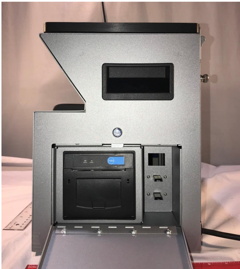
SS2043 Clear Ballot Group, Inc. Vote Visualization System, Model ClearCast Printer with Locked Access Panel Opened
