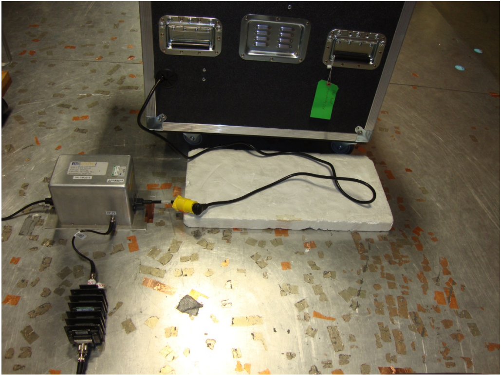
Figure E1. Conducted RF Immunity Test Setup – AC Mains
