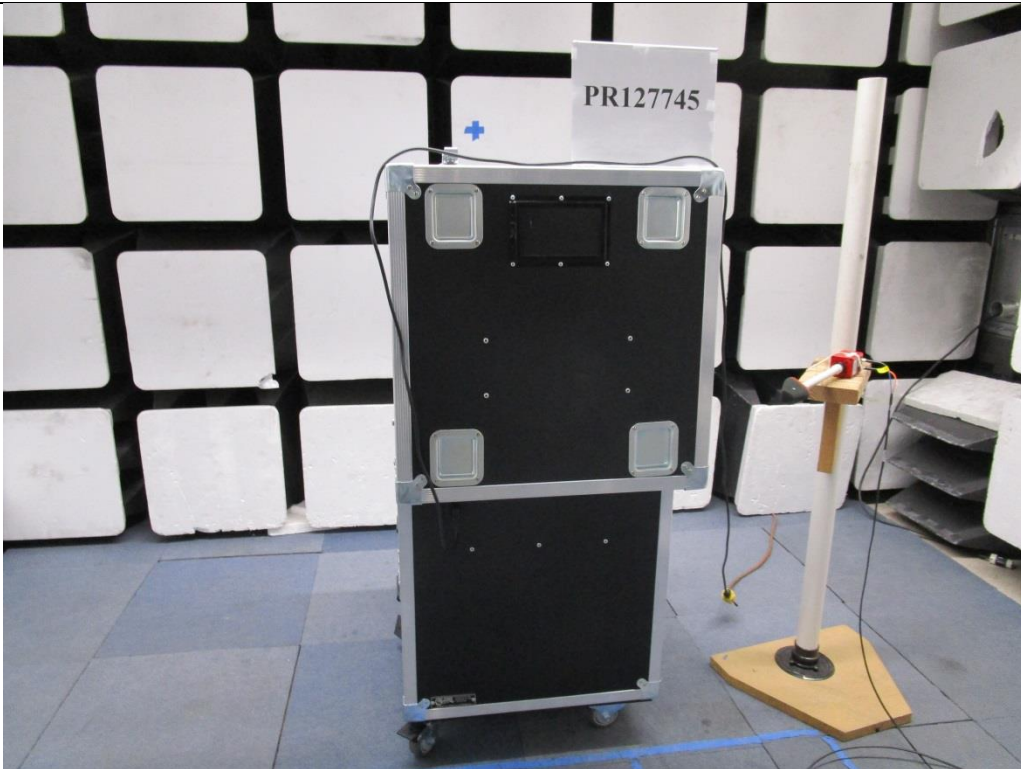
Figure B3. Radiated RF Immunity Test Setup –Back Side.
