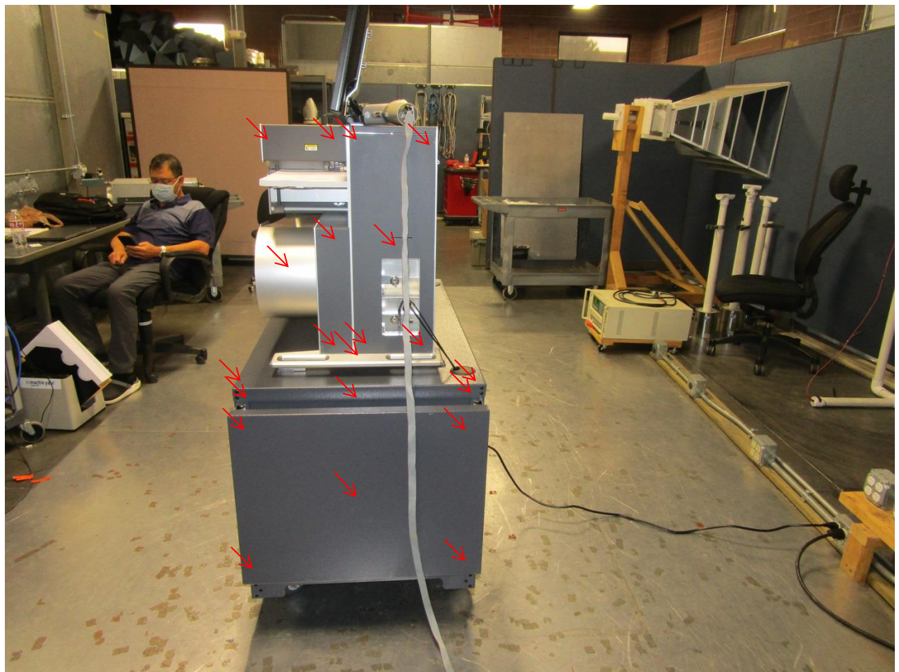
Figure A3. Electrostatic Discharge Test Setup.
