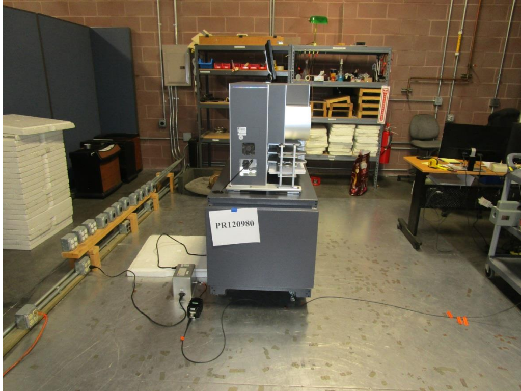
Figure E1. Conducted RF Immunity Test Setup.
