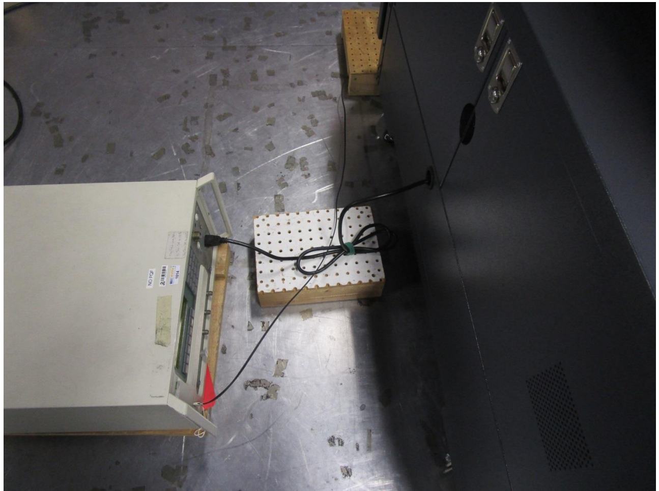
Figure D2. Surge Immunity Test Setup – AC Mains.
