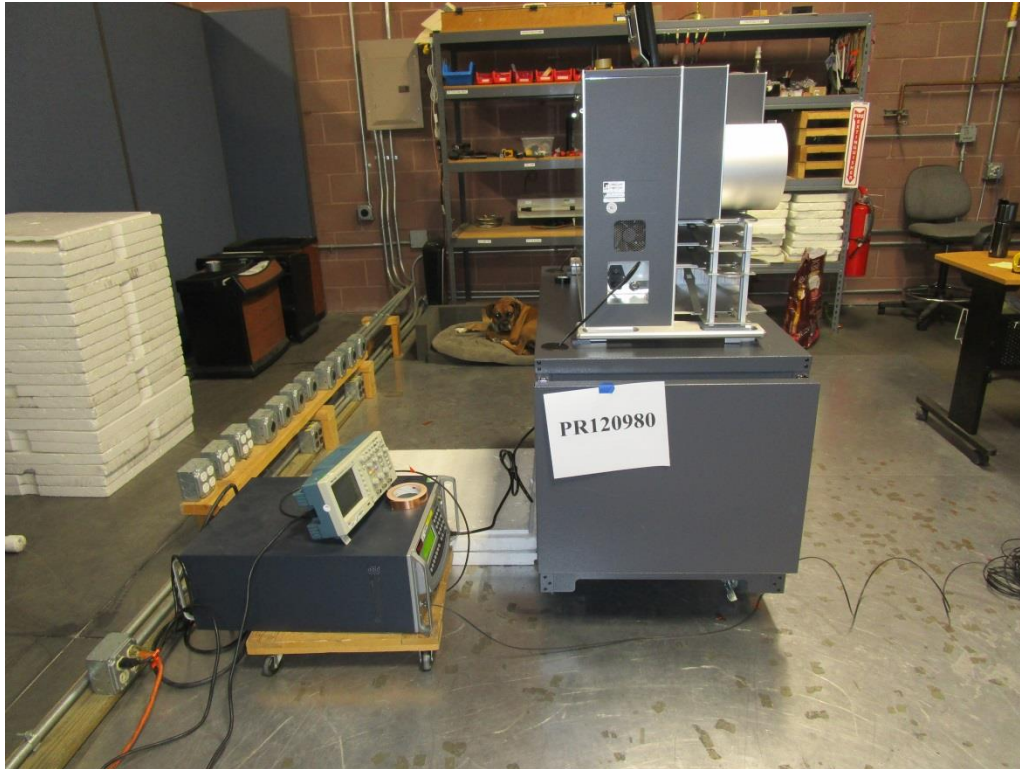
Figure C1. Electrical Fast Transient Test Setup.
