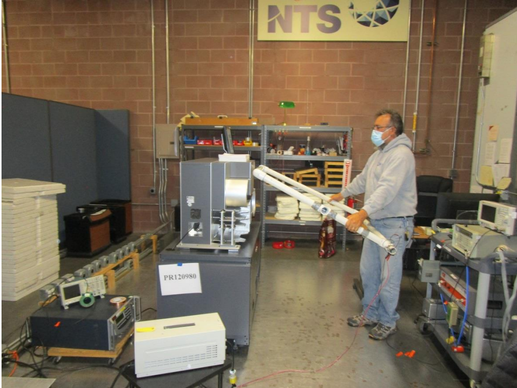
Figure F1. Power Frequency H-field Immunity Test Setup.
