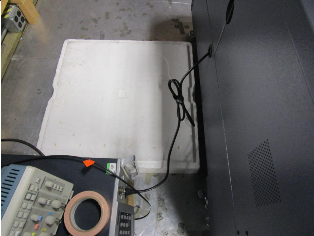
Figure C2. Electrical Fast Transient Test Setup – AC Mains.
