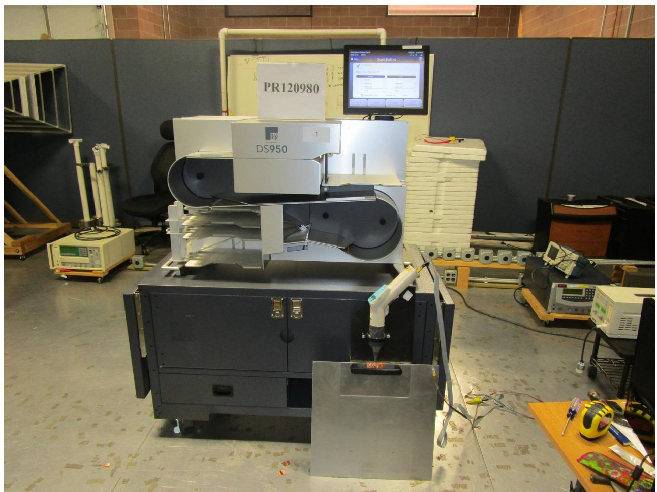
Figure A1. Electrostatic Discharge Test Setup.
