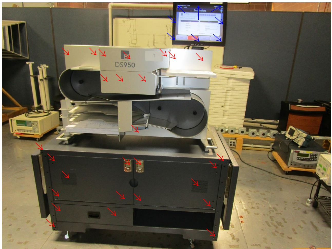
Figure A2. Electrostatic Discharge Test Setup.
