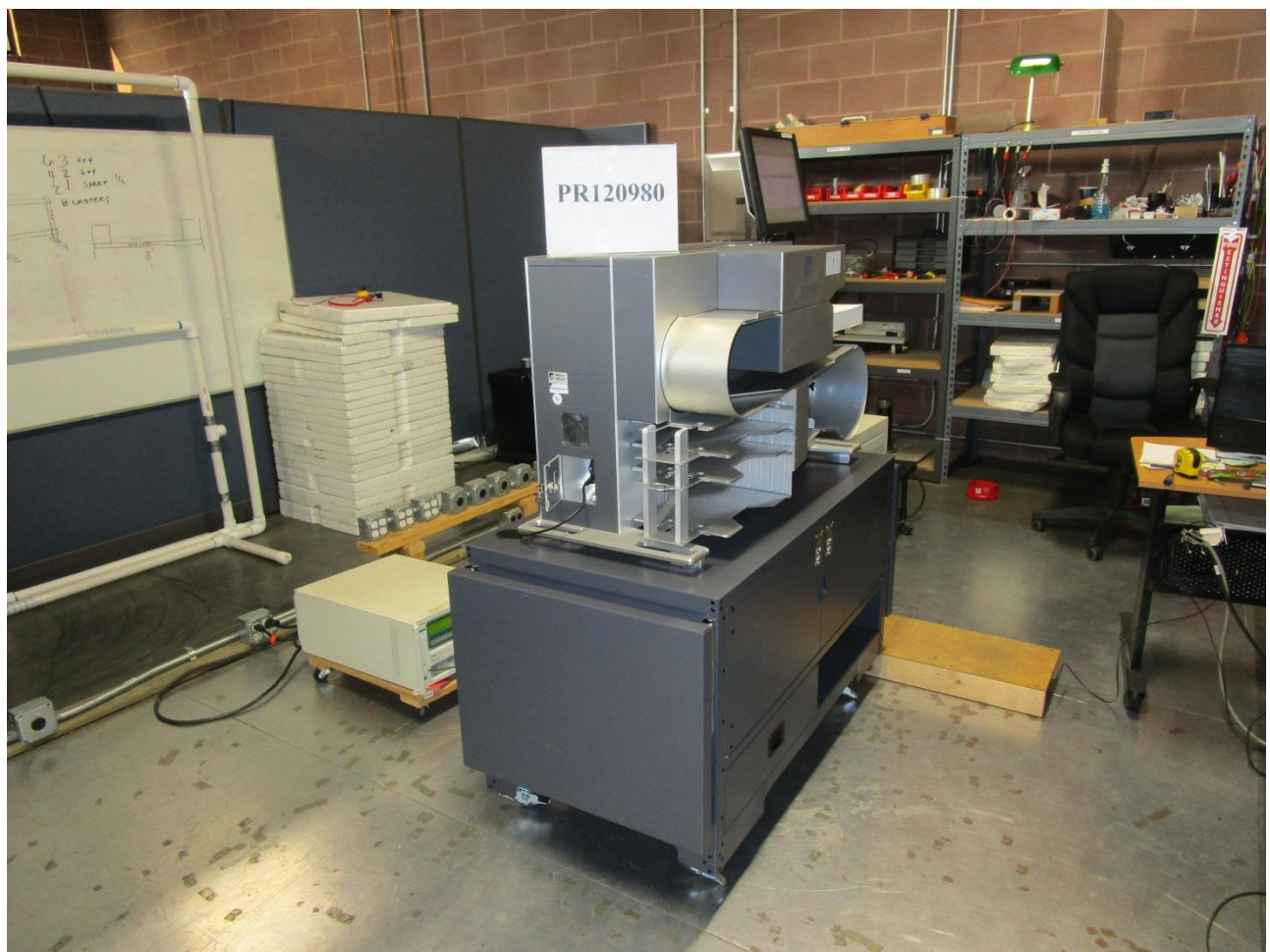
Figure D1. Surge Immunity Test Setup.
