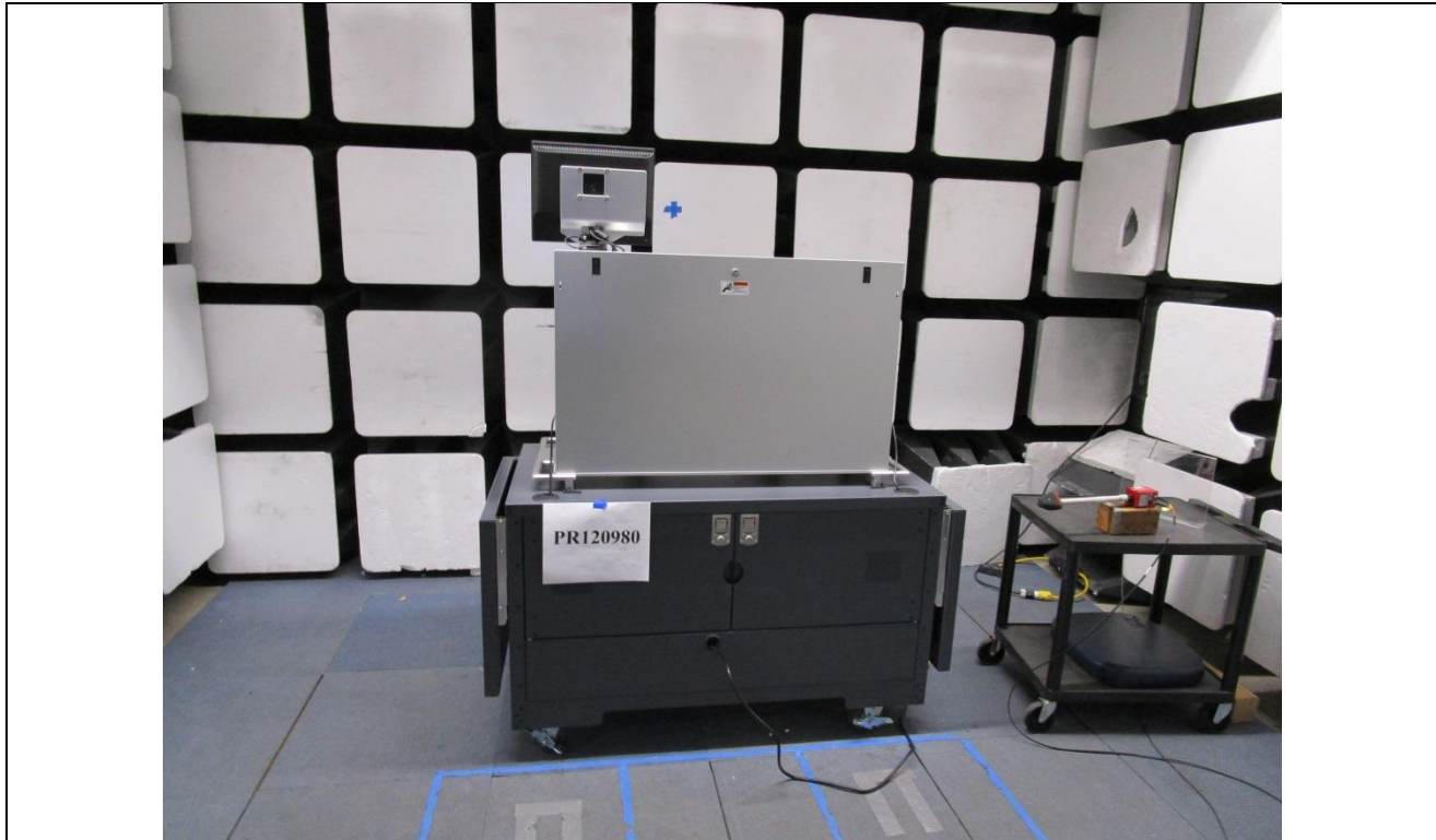
Figure B3. Radiated RF Immunity Test Setup – Back Side.
