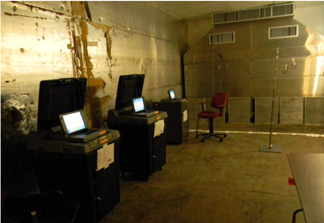
Photograph 24: ES&S FL EVS 4.5.0.0 Temperature and Power Variation
