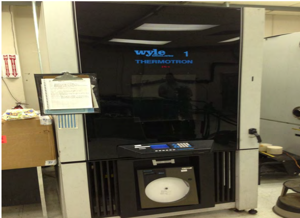
Photograph 32: ES&S FL EVS 4.5.0.0 High Temperature
