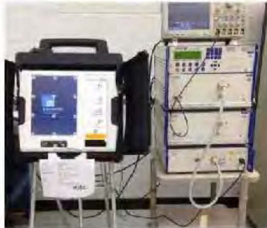
Photograph No. 12: ES&S BL ENS 4.50.01 lightning Surge
