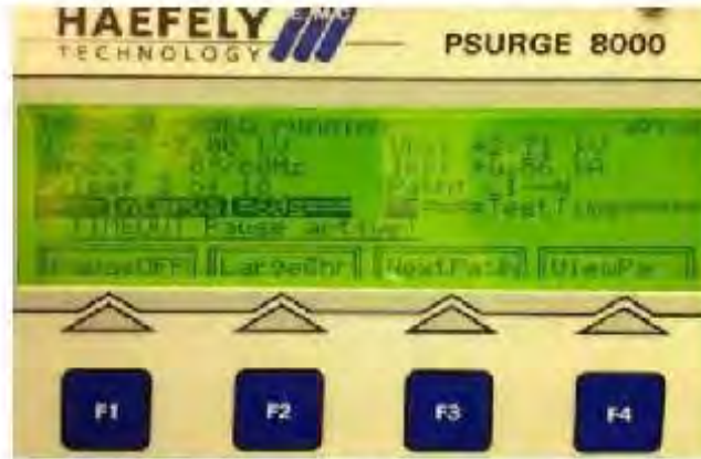
Photograph No. 11: ES&S BL ENS 4.50.01 lightning Surge
