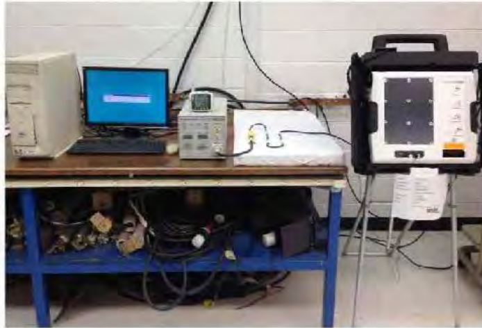
Photograph No. 21: ES&S FL EVS 4.5.0.0 Electrical Power Disturbance
