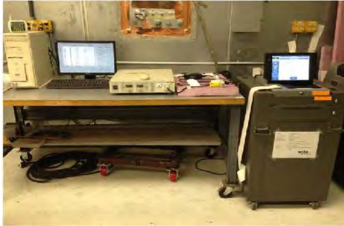
Photograph 19: ES&S FL EVS 4.5.0.0 Electrical Power Disturbance
