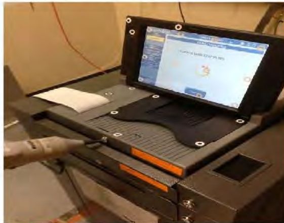
Photograph 18: ES&S FL EVS 4.5.0.0 Electrostatic Disruption
