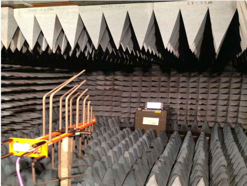
Photograph 22: ES&S FL EVS 4.5.0.0 Electromagnetic Susceptibility
