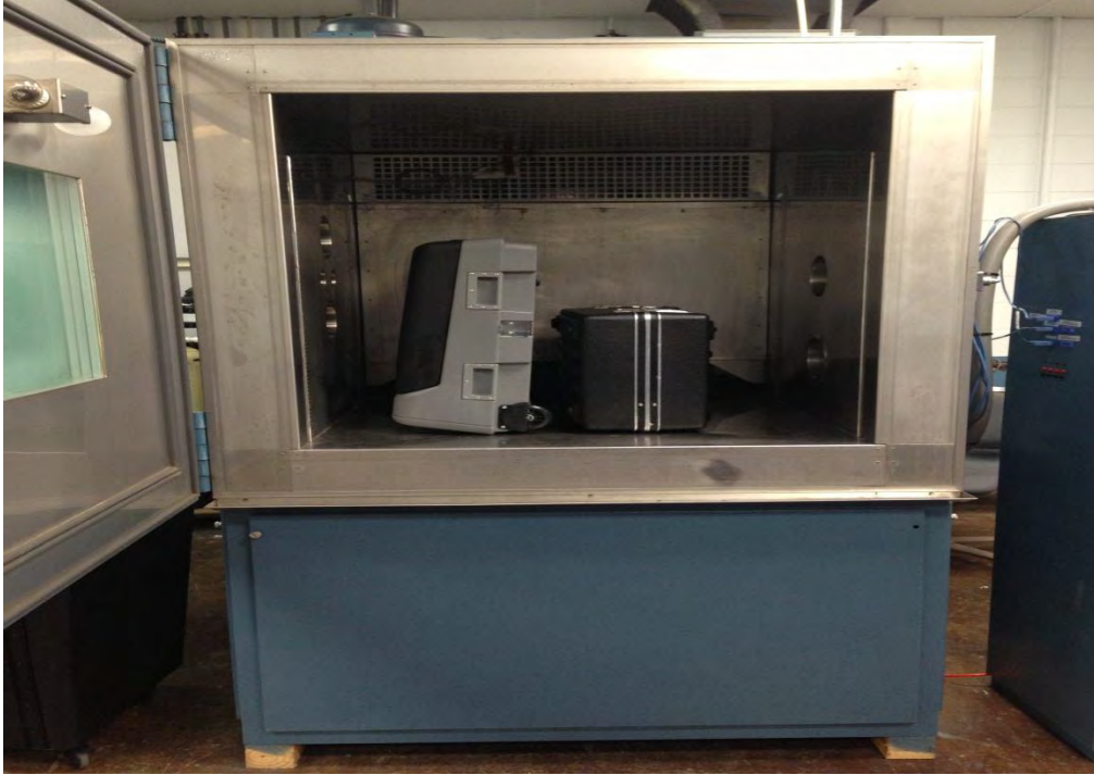
Photograph 29: ES&S FL EVS 4.5.0.0 Low Temperature
